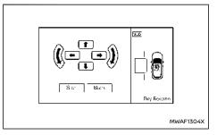
Depress the brake pedal and stop the vehicle, then touch the parking guide box adjustment icon (△▽) on the screen.
