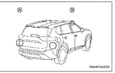
The two radar sensors (A) for the Intelligent Blind Spot Intervention system are located near the rear bumper. Always keep the area near the radar sensors clean. The radar sensors may be blocked by temporary ambient conditions such as splashing water, mist or fog.
