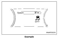
To turn off the ESP system, perform the following steps in the vehicle information display.
