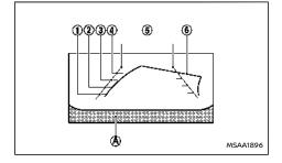
Guiding lines which indicate the vehicle width and distances to objects with reference to the bumper line A are displayed on the monitor.
