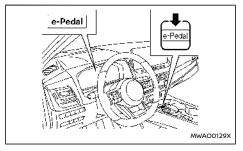
The e-Pedal Step system will be turned ON or OFF each time the <e-Pedal> switch (located on the centre console) is operated. (The e-Pedal indicator in the vehicle information display shows the status of the e-Pedal Step system.)
