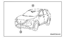
The Intelligent Emergency Braking with Pedestrian Detection system uses a radar sensor (2) located on the front of the vehicle to measure the distance to the vehicle ahead in the same lane.
