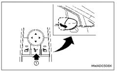
The outside rearview mirror remote control operates when the power switch is in the ON position.
