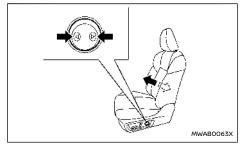
Push the adjusting switch as shown to adjust the seat lumbar area until the desired position is achieved.
