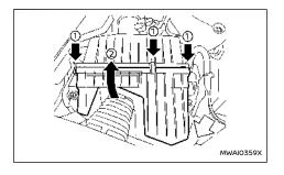
Operating the engine with the air cleaner filter off can cause you or others to be burned. The air cleaner filter not only cleans the intake air, it also stops flame if the engine backfires. If the air cleaner filter is not installed and the engine backfires, you could be burned. Never drive with the air cleaner filter off. Be cautious working on the engine when the air cleaner filter is off.
