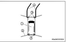
The bird's-eye view shows the overhead view of the vehicle which helps confirm the vehicle position and the predictive course to a parking space.
