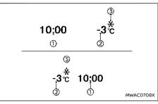
The clock 1 and outside air temperature 2 are displayed on the upper side of the vehicle information display.
