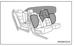
The supplemental side-impact air bag is located at the outside of the front seats' seatbacks.
