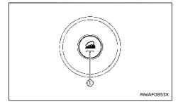
When additional braking is required on steep downhill roads, activate the hill descent control system by pushing the hill descent control switch on.
