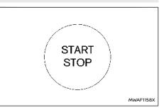
When the power switch is pushed without depressing the brake pedal, the power switch will illuminate.
