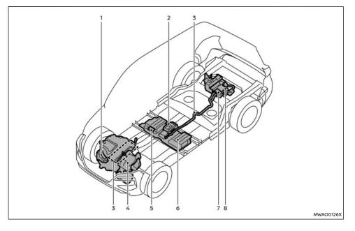
The e-POWER system consists of the following high voltage parts.
