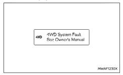
If the [4WD System Fault See Owner's Manual] warning appears, there may be a malfunction in the 4WD system. Reduce vehicle speed and have your vehicle checked by a NISSAN dealer or qualified workshop as soon as possible.
