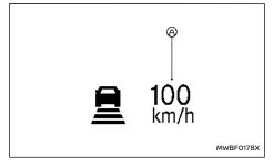
The driver can override ICC by depressing the accelerator pedal. The set speed indicator (A) will flash when the vehicle speed exceeds the set speed. The vehicle detect indicator will turn off when the area ahead of the vehicle is open. When the pedal is released, the vehicle will return to the previously set speed.
