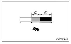
The ECO Pedal Guide display can be selected in the vehicle information display in the ECO mode. (See "4. [ECO Pedal Guide]" (P.115).) Use the ECO Pedal Guide function for improving fuel economy.
