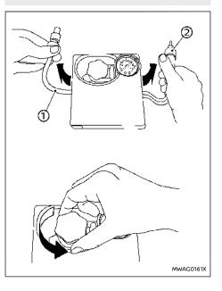
Take the hose ① and the power plug ② out of the air compressor. Remove the cap of the bottle holder from the air compressor.
