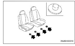
This vehicle includes front floor mat brackets to act as a floor mat positioning aid. Genuine NISSAN floor mats have been specially designed for your vehicle model. Position the mat by placing the floor mat bracket hook(s) through the floor mat grommet hole while centering the mat in the foot area.
