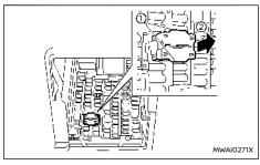
The extended storage switch is used when shipping the vehicle. It is located in the fuse panel. If any electrical equipment does not operate, ensure the extended storage switch is pushed fully in place.
