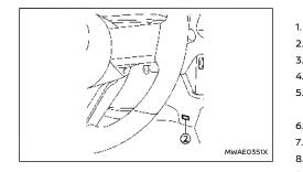
The sensors (1) and (2), located on the instrument panel, help maintain a constant temperature. Do not put anything on or around the sensors.
