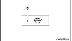
The rear window wiper and washer operate when the power switch is in the ON position.
