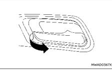
To unlock and open the door, pull the inside door handle as illustrated.
