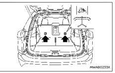
Anchorages are located as illustrated. Position the top tether strap over the top of the seatback and secure it to the tether anchorage that provides the straightest installation. Tighten the tether strap according to the manufacturer's instruction to remove any slack.
