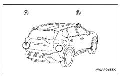
The Intelligent Blind Spot Intervention system uses radar sensors (a) installed near the rear bumper to detect other vehicles in an adjacent lane. In addition to the radar sensors, the Intelligent Blind Spot Intervention system uses a camera (b) installed behind the windscreen to monitor the lane markers of your travelling lane.
