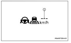
When the **<CANCEL>** switch is pushed down to SET- under the following conditions, the ProPILOT Assist system cannot be set and the vehicle set speed indicator ① blinks for approximately 2 seconds:
