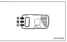
The cargo light has a three-position switch.
