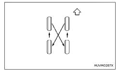
NISSAN recommends that tyres be rotated every 5,000 km (3,000 miles) for Four-Wheel Drive (4WD) or every 10,000 km (6,000 miles) for Two-Wheel Drive (2WD) model. However, the timing for tyre rotation may vary according to your driving habits and the road surface conditions. (See "Flat tyre" (P.403) for the tyre replacement.)
