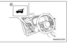
Power back door switch — Instrument panel
