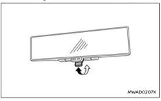
The mode can be switched when the power switch is in the ON position.
