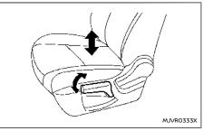
Pull up or push down the adjusting lever to adjust the seat height until the desired position is achieved.
