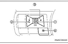
The vehicle information display can be changed using the scroll dial (1), 2 (2), and 4 (3) located on the steering wheel.
