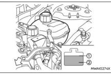
Check the coolant level **in the reservoir when the engine is cold.** If the coolant level is below the MIN
