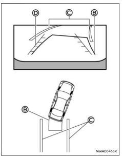
When the vehicle is parked in the space completely, place the shift position in the P (Park) position and apply the parking brake.
