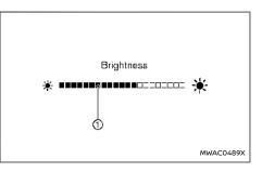
The instrument brightness control switch can be operated when the power switch is in the ON position. When the switch is operated, the vehicle information display switches to the brightness adjustment mode.
