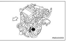
The engine serial numbers are located as shown.
