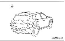
The two radar sensors (a) for the BSW system are located near the rear bumper. Always keep the area near the radar sensors clean.
