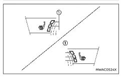
The front seats are warmed by built-in heaters. The switches are located on the instrument panel and can be operated independently of each other.
