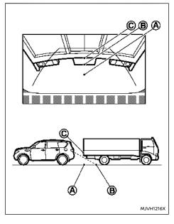
The position  $\bigcirc$  is shown farther than the position B in the display. However, the position D is actually at the same distance as the position A. The vehicle may hit the object when reversing to the position A if the object projects over the actual moving course.
