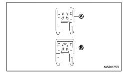
If the fuse is open (a), replace it with a new fuse (B).  If a new fuse also opens, have the electrical system checked and repaired. It is recommended you visit a NISSAN dealer or qualified workshop for this service.
