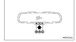
The inside rearview mirror is designed so that it automatically changes reflection according to the intensity of the headlights of the following vehicle. The anti-glare system will be automatically turned on when the power switch is placed in the ON position.
