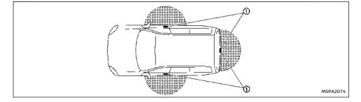
The Intelligent Key functions can only be used when the Intelligent Key is within the specified operating range from the lock or capacitive unlock sensors/request switch ①.
