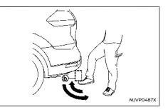
The back door can be operated using a quick kicking motion under the centre of the rear bumper.
