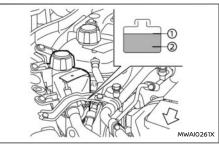
Check the coolant level in the reservoir when the engine is cold. If the coolant level is below the MIN level (2), add coolant to the MAX level (1).
