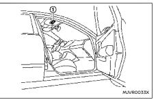
Warning labels about the supplemental air bag system are placed in the vehicle as shown in the illustration.
