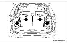
Before folding the third row seats, secure the outer seat belt on the seat belt hook. (See "Seat belt hooks" (P.42).)
