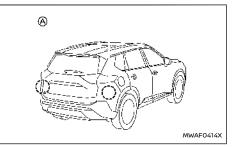
The BSW system uses radar sensors (A) installed near the rear bumper to detect other vehicles in an adjacent lane.
