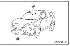
The radar sensor B is located on the front of the vehicle. The camera A is located on the upper side of the windscreen.
