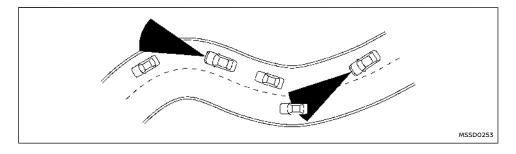
When driving on some roads, such as winding, hilly, curved, narrow roads, or roads which are under construction, the radar sensor may detect vehicles in a different lane, or may temporarily not detect a vehicle travelling ahead. This may cause the ICC system to decelerate or accelerate the vehicle.
