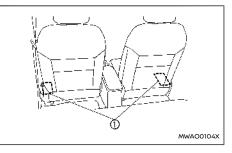
The air inlets 1 for cooling the Lithium ion (Li-ion) battery are located under the front seats.
