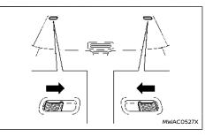
Before moving the rear (outer) luggage board, release the lock on the both sides of the board as shown (where fitted).
