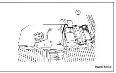
The 12-volt battery (1) is located on the luggage room. To access the 12-volt battery, raise the luggage floor board and remove the tool holder (s).
