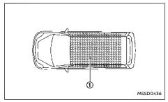
The Intelligent Key can only be used for starting the e-POWER system when the Intelligent Key is within the specified operating range 1 as illustrated.
