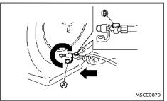
5. Remove the protective cap (a) of the hose and screw the hose securely onto the tyre valve. Make sure that the pressure release valve (a) is securely tightened. Make sure that the air compressor switch is in the OFF (O) position, and then insert its power plug into the power outlet in the vehicle.
