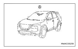
The Traffic Sign Recognition (TSR) system provides the driver with information about the most recently detected speed limit. The system captures the road sign information with the multi-sensing front camera unit (a) located on the windshield in front of the inside rearview mirror and displays the detected signs in the vehicle information display and in the Head Up Display (HUD) (where fitted). (See "Head Up Display (HUD) (where fitted)" (P.118).)
