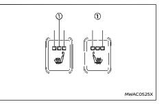
The second row seats are warmed by built-in heaters. The switches are located on the back of the centre console and can be operated independently of each other.
