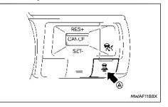
The distance to the vehicle ahead can be selected at the time of the ICC standby or the ICC is active.
