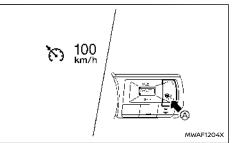
To turn on the conventional (fixed speed) cruise control mode, push and hold the Cruise ON/OFF switch (A) for longer than about 1.5 seconds.
