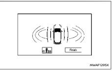
When the vehicle speed becomes approximately 10 km/h (6 MPH) or higher while parking position detection is in progress, the screen changes. When the vehicle speed drops to approximately 10 km/h
