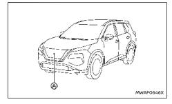
The radar sensor  $\textcircled{}{}$  is located on the front of the vehicle.
