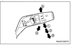
The windscreen wiper and washer operates when the power switch is in the ON position.
