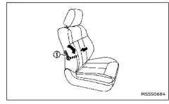
Pull or push the adjusting lever (1) to adjust the seat lumbar area until the desired position is achieved.
