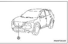
The sensor for the ICC system  $\textcircled{\ensuremath{B}}$  is located on the front of the vehicle.
