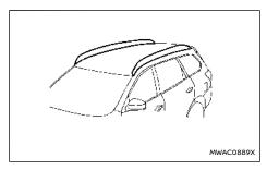
Do not apply any load directly to the roof side rails. Cross bars must be installed before applying load/ cargo/luggage to the roof of the vehicle. For additional information, it is recommended that you contact a NISSAN dealer or qualified workshop.
