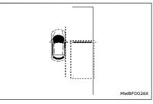
Drive slowly forward and depress the brake pedal to stop the vehicle when parallel to the parking position.
