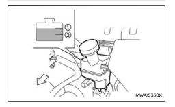
Check the fluid level in the reservoir. If the fluid is below the MIN line Q, the brake warning light will illuminate. Add fluid up to the MAX line D. (See
