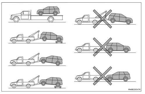
NISSAN recommends that your vehicle be towed with the driving (front) wheels off the ground or place the vehicle on a flat bed truck as illustrated.
