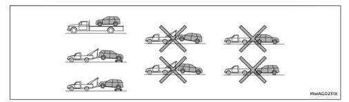
NISSAN recommends that towing dollies be used when towing your vehicle or the vehicle be placed on a flat bed truck as illustrated.
