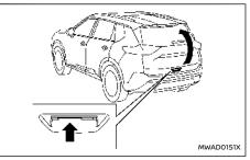
To open the back door, unlock it. Pull up the back door to open.
