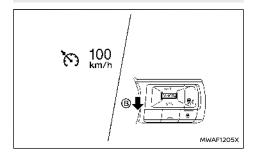
To set cruising speed, accelerate your vehicle to the desired speed, push down the **<CANCEL>** switch to SET- (B) and release it. (The colour of the cruise indicator changes to green and vehicle set speed indicator comes on.) Take your foot off the accelerator pedal. Your vehicle will maintain the set speed.
