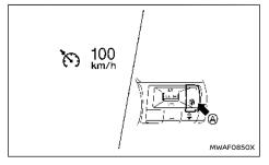
To turn on the conventional (fixed speed) cruise control mode, push and hold the ProPILOT Assist switch (A) for longer than about 1.5 seconds.
