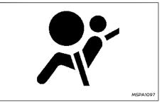
The supplemental air bag warning light, displaying real in the meter monitors the circuits for the air bag systems, pre-tensioner seat belt system and all related wiring.
