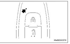
The light blinks only when you push any button on the Intelligent Key. The light illumination only signifies that the Intelligent Key has transmitted a signal. You may look and/or listen to verify that the vehicle has performed the intended operation. If the light does not blink, your battery may be too weak to communicate to the vehicle. If this occurs, the battery may need to be replaced.
