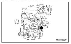
The engine serial numbers are located as shown.
