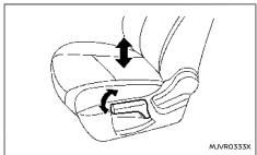
Pull up or push down the adjusting lever to adjust the seat height until the desired position is achieved.
