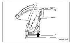
The vehicle identification plate is affixed as shown (on the driver's side).
