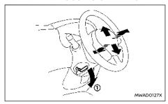
Pull the lock lever 1 down and adjust the steering wheel up, down, forward or rearward to the
