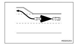
When driving on the highway at a vehicle set speed and approaching a slower travelling vehicle ahead, the ICC system adjusts the speed to maintain the distance, selected by the driver, from the vehicle ahead. If the vehicle ahead changes lanes or exits the highway, the ICC system accelerates and maintains the vehicle set speed. Pay attention to the driving operation to maintain control of the vehicle as it accelerates to the set speed.
