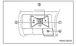
The vehicle information display can be changed using the scroll dial (1),  $\stackrel{\bullet}{\longrightarrow}$  (2), and  $\stackrel{\bullet}{\blacktriangleleft}$ located on the steering wheel.
