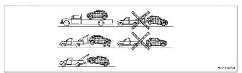
NISSAN recommends that your vehicle be towed with the driving (front) wheels off the ground or place the vehicle on a flat bed truck as illustrated.
