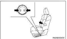
Push the adjusting switch as shown to adjust the seat lumbar area until the desired position is achieved
