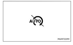
This indicator is displayed when the vehicle is stopped if the engine is prevented from automatically stopping by the Stop/Start System under the inhibition conditions. See "Stop/Start System" (P.235).
