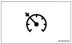
When the system is not operating properly, the chime sounds and the colour of the cruise indicator will change to yellow.
