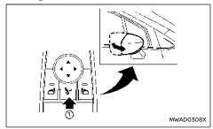
The outside rearview mirror remote control operates when the ignition switch is in the ON position.
