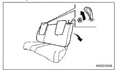
Pull the strap (A) and position the seatback at the desired angle. Release the strap after positioning the seat at the desired angle.
