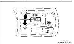
The vehicle set speed can be adjusted.
