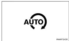
This indicator is displayed when the Stop/Start System is activated.
