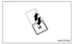
The passenger's switch can control its corresponding window. When the window lock button on the driver's switch is pushed, the rear passenger's switch cannot be operated.
