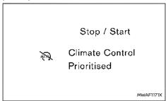
When the vehicle is stopped, the guidance is displayed if the Stop/Start system is deactivated since the air conditioner (cooling, heating or dehumidifying functions) is given priority.
