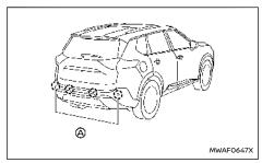
The parking sensors (A) are located on the rear bumper. Observe the following items to ensure proper operation of the system:
