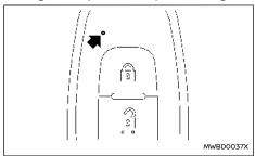
The light blinks only when you push any button on the Intelligent Key. The light illumination only signifies that the Intelligent Key has transmitted a signal. You may look and/or listen to verify that the vehicle has performed the intended operation. If the light does not blink, your battery may be too weak to communicate to the vehicle. If this occurs, the battery may need to be replaced.
