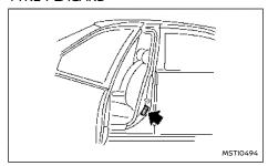
The cold tyre pressures are shown on the tyre placard affixed to the driver's side centre pillar.
