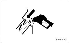
The fuel tank is not equipped with a fuel-filler cap. After opening the fuel-filler lid, insert the fuel pump nozzle directly into the fuel-filler opening. When the fuel pump nozzle is pulled out, the fuel-filler opening will be sealed.
