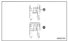
If the fuse is open (a), replace it with a new fuse (b).
