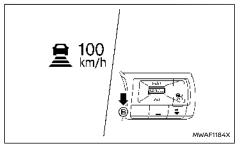
To set cruising speed, accelerate your vehicle to the desired speed, push down the <CANCEL> switch to <SET-> (B) and release it. (The ICC system) ON indicator (green), set distance indicator and set vehicle speed indicator come on.) Take your foot off the accelerator pedal. Your vehicle will maintain the set speed.
