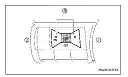
Switches for the trip computer are located on the left side of the steering wheel.
