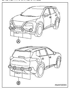
The parking sensors (a) (where fitted) and (b) are located on the bumpers.
