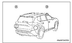
The two radar sensors (A) for the Intelligent Blind Spot Intervention system are located near the rear bumper. Always keep the area near the radar sensors clean
