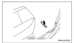
The vehicle identification number is located as shown.
