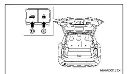
Power back door close and lock switches — Back
