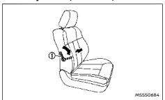
Pull or push the adjusting lever 10 to adjust the seat lumbar area until the desired position is achieved.
