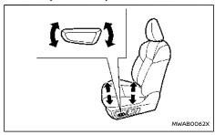
Move the switch as shown to adjust the angle of the front portion or height of the seat.
