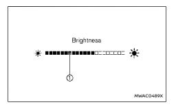
The instrument brightness control switch can be operated when the ignition switch is in the ON position. When the switch is operated, the vehicle information display switches to the brightness adjustment mode.
