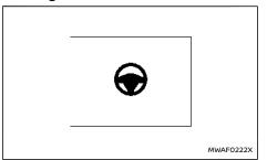
The Steering Assist switch is used to temporarily turn on and off the Steering Assist system.
