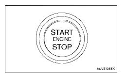
When the ignition switch is pushed without depressing the brake pedal, the ignition switch will illuminate.
