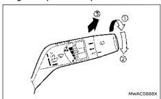
The rear window wiper and washer operate when the ignition switch is in the ON position.
