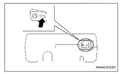
6. Place the ignition switch in the ON position. Then turn the compressor switch to the ON (-) position and inflate the tyre up to the pressure that is specified on the tyre placard affixed to the driver's side centre pillar if possible, or to the minimum of 180 kPa (26 psi). Turn the air compressor off briefly in order to check the tyre pressure with the pressure gauge.
