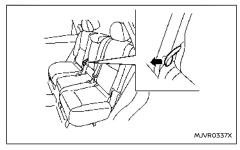
Pull the strap to unlatch the seatback and fold it down until it is horizontal.
