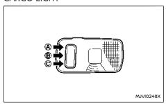
The cargo light has a three-position switch.
