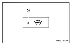
The heated windscreen button is located on the front air conditioner control panel.
