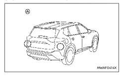
The two radar sensors (A) for the RCTA system are located near the rear bumper. Always keep the area near the radar sensors clean
