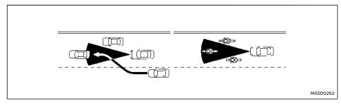
The detection zone of the radar sensor is limited. A vehicle ahead must be in the detection zone for the vehicle-to-vehicle distance detection mode to maintain the selected distance from the vehicle ahead.
