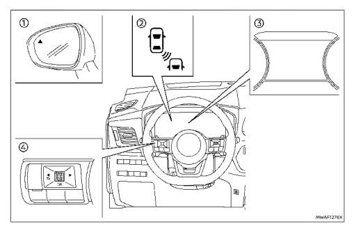
indicator continue to flash until the detected vehicle leaves the detection zone.
