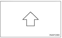
Gear Shift Indicator appears in the transmission position indicator when the driver should shift into a higher gear as indicated by the up arrow.
