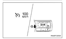
To set cruising speed, accelerate your vehicle to the desired speed, push down the <CANCEL> switch to <SET->(B) switch and release it. (The colour of the cruise indicator changes to green and vehicle set speed indicator comes on.) Take your foot off the accelerator pedal. Your vehicle will maintain the set speed.
