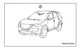
The Traffic Sign Recognition (TSR) system provides the driver with information about the most recently detected speed limit. The system captures the road sign information with the multi-sensing front camera unit (A) located on the windscreen in front of the inside rearview mirror and displays the detected signs in the vehicle information display and in the Head Up Display (HUD) (where fitted). (See "Head Up Display (HUD) (where fitted)" (P.102).)
