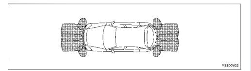
The parking sensor (sonar) system sounds a tone to inform the driver of obstacles near the bumper. When the parking sensor (sonar) system is turned on, the parking sensor (sonar) view will automatically appear in the vehicle information display.
