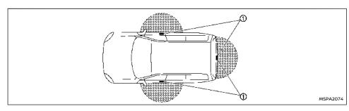
The Intelligent Key functions can only be used when the Intelligent Key is within the specified operating range from the lock or capacitive unlock sensors/request switch (1).
