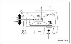
The system is operated by the Cruise ON/OFF switch and four control switches, all mounted on the steering wheel.
