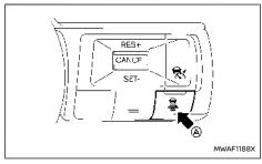
at the time of the ICC standby or the ICC is active. Each time the DISTANCE switch (A) is pushed, the set distance will change to long, middle, short and back to long again in that sequence.
