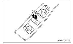
The driver's switch, the main switch, can control all windows
