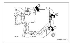
To remove the filter, release the lock pins ① and pull the unit upward ②.
