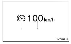
The speed limiter operating condition is shown on the vehicle information display.
