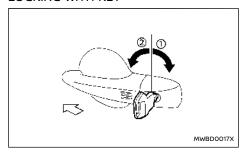
To lock the driver's door, turn the driver's door key cylinder to the rear of the vehicle (1).
