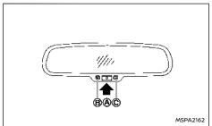
The inside rearview mirror is designed so that it automatically changes reflection according to the intensity of the headlights of the following vehicle. The anti-glare system will be automatically turned on when the ignition switch is placed in the ON position.
