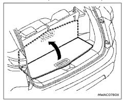
To use the vertical mode, insert the luggage board to slit of the finisher.
