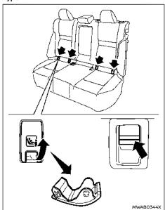
The ISOFIX lower anchor points are located under covers labelled ISOFIX at the bottom of the rear seat cushions. To access a ISOFIX lower anchor point, insert your finger into the cover and pull the cover off.
