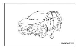
To display the multiple views, the Intelligent Around View Monitor system uses cameras (1) located on the front grille, on the vehicle's outside rearview mirrors and one just above the vehicle's rear number plate.
