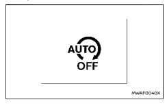
The system can be temporarily deactivated by pressing the Stop/Start OFF switch. Pressing the switch again or restarting the engine by using the ignition switch will reactivate the Stop/Start System.
