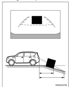
When reversing the vehicle down a hill, the distance guide lines and the vehicle width guide lines are shown farther than the actual distance. Note that any object on the hill is closer than it appears on the monitor.
