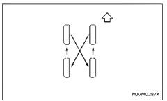
NISSAN recommends that tyres be rotated every 10,000 km (6,000 miles). However, the timing for tyre rotation may vary according to your driving habits and the road surface conditions. (See "Jacking up vehicle and replacing tyres" (P.425) for the tyre replacement.)
