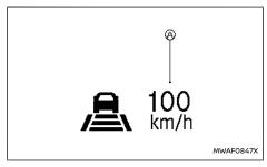
When passing another vehicle, the vehicle set speed indicator (A) flashes when the vehicle speed exceeds the set speed. The vehicle ahead detection indicator turns off when the area ahead of the vehicle is open. When the pedal is released, the vehicle returns to the previously set speed. Even though your vehicle speed is set in the ICC system,
