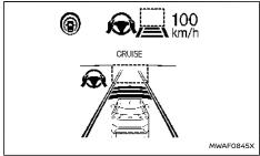
System set display - no vehicle detected ahead\*
