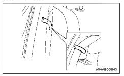
When folding down the second row seats, hook the second row outer seat belts on the seat belt hooks.
