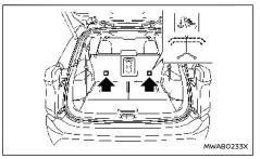
Anchorages are located as illustrated. Position the top tether strap over the top of the seatback and secure it to the tether anchorage that provides the straightest installation. Tighten the tether strap according to the manufacturer's instruction to remove any slack.
