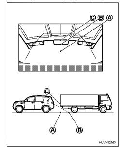
The position © is shown farther than the position B in the display. However, the position C is actually at the same distance as the position (A). The vehicle may hit the object when reversing to the position (a) if the object projects over the actual reversing course.
