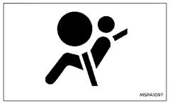
The supplemental air bag warning light, displaying 🖈 in the meter monitors the circuits for the air bag systems, pre-tensioner seat belt system and all related wiring.
