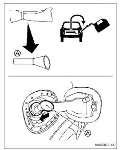
If you need to refuel from a portable fuel container, use the funnel (A) stored in the tool bag (located under the luggage board).
