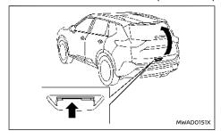
To open the back door, unlock it. Pull up the back door to open.
