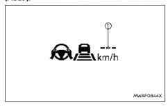
When the **<CANCEL>** switch is pushed down to **<SET->** under the following conditions, the ProPLOT Assist system cannot be set and the vehicle set speed indicator ① blinks for approximately 2 seconds:
