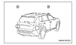
The Intelligent Blind Spot Intervention system uses radar sensors (a) installed near the rear bumper to detect other vehicles in an adjacent lane. In addition to the radar sensors, the Intelligent Blind Spot Intervention system uses a camera (a) installed behind the windscreen to monitor the lane markers of your travelling lane.
