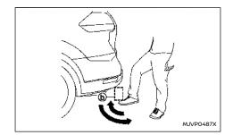
The back door can be operated using a quick kicking motion under the centre of the rear bumper.
