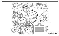
Check the coolant level in the reservoir when the engine is cold. If the coolant level is below the MIN
