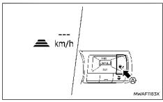
To turn on the cruise control, quickly push and release the Cruise ON/OFF switch (A). The ICC system ON indicator (grey), set distance indicator and set vehicle speed indicator come on and in a standby state for setting.
