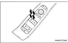
The automatic function enables a window to fully open or close without holding the switch down or up.
