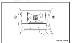
To change the status of the Driving Aids, use (1) or (2) to navigate the settings screen. For additional information, see "How to use the vehicle information display" (P.82).
