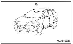
The ambient image sensor (A) for the adaptive LED headlight system is located in front of the inside rearview mirror. To keep the proper operation of the adaptive LED headlight system and prevent a system malfunction, be sure to observe the following:
