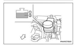
Check the fluid level in the reservoir. If the fluid is below the MIN line ②, the brake warning light will illuminate. Add fluid up to the MAX line ①. (See
