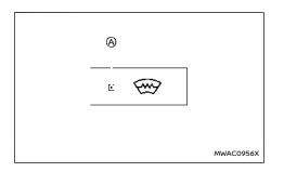
The heated windscreen button is located on the front air conditioner control panel.
