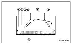
Guiding lines which indicate the vehicle width and distances to objects with reference to the bumper line (A) are displayed on the monitor.
