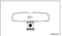
The inside rearview mirror is designed so that it automatically changes reflection according to the intensity of the headlights of the following vehicle.
