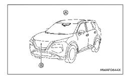
The Intelligent Emergency Braking with Pedestrian Detection system uses a radar sensor (B) located on the front of the vehicle to measure the distance to the vehicle ahead in the same lane.
