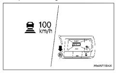
To set cruising speed, accelerate your vehicle to the desired speed, push the <SET-> switch (B) and
