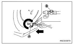
5. Remove the protective cap (A) of the hose and screw the hose securely onto the tyre valve. Make sure that the pressure release valve (B) is securely tightened. Make sure that the air compressor switch is in the OFF (()) position, and then insert its power plug into the power outlet in the vehicle.
