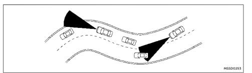
When driving on some roads, such as winding, hilly, curved, narrow roads, or roads which are under construction or on a slope, the sensor may detect vehicles in a different lane, or may temporarily not detect a vehicle travelling ahead. This may cause the system to work inappropriately.
