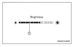
The instrument brightness control switch can be operated when the ignition switch is in the ON position. When the switch is operated, the vehicle information display switches to the brightness adjustment mode.
