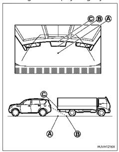
The position  $\bigcirc$  is shown farther than the position  $\bigcirc$  in the display. However, the position  $\bigcirc$  is actually at the same distance as the position  $\bigcirc$  . The vehicle may hit the object when reversing to the position  $\bigcirc$  if the object projects over the actual moving course.
