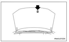
The air conditioner specification label is attached to the underside of the bonnet as shown
