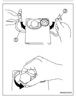
2. Take the hose ① and the power plug ② out of the air compressor. Remove the cap of the bottle holder from the air compressor.
