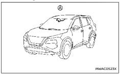
The ambient image sensor (A) for the high beam assist system is located in front of the inside rearview mirror. To keep the proper operation of the high beam assist system and prevent a system malfunction, be sure to observe the following:
