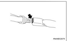
The centre seat belt buckle is identified by the CENTER mark. The centre seat belt tongue can be fastened only into the centre seat belt buckle.
