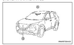
The radar sensor (B) is located on the front of the vehicle. The camera (a) is located on the upper side of the windscreen
