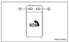
The indicator lights ① and ② above the SOS button indicate the status of the vehicle emergency call system. If the indicator light is illuminated red or no indicator light is illuminated the emergency call may not connect to the emergency call centre when the SOS button is pressed. Also an intelligent Emergency call may not be sent when a collision occurs.
