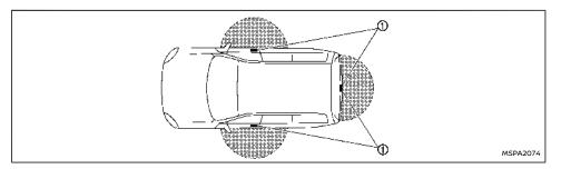
The Intelligent Key functions can only be used when the Intelligent Key is within the specified operating range from the lock or capacitive unlock sensors/request switch ①.
