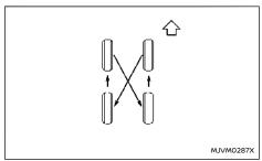
NISSAN recommends that tyres be rotated every 10,000 km (6,000 miles). However, the timing for tyre rotation may vary according to your driving habits and the road surface conditions. (See "Jacking up vehicle and replacing tyres" (P.448) for the tyre replacement.)
