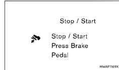
When the vehicle is stopped, the guidance is displayed if the Stop/Start system is deactivated due to not fully depressing the brake pedal.
