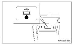
The USB connection port is located on the lower part of the instrument panel. Insert USB devices or iPod connectors into this port.
