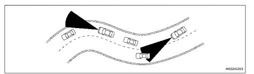
When driving on some roads, such as winding, hilly, curved, narrow roads, or roads which are under construction, the radar sensor may detect vehicles in a different lane, or may temporarily not detect a vehicle travelling ahead. This may cause the ICC system to decelerate or accelerate the vehicle.
