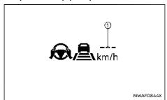
When the <SET-> switch is pushed down under the following conditions, the ProPILOT Assist system cannot be set and the vehicle set speed indicator (1) blinks for approximately 2 seconds:
