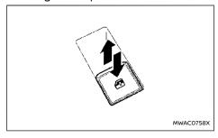
The passenger's switch can control its corresponding window. When the window lock button on the driver's switch is pushed, the rear passenger's switch cannot be operated.
