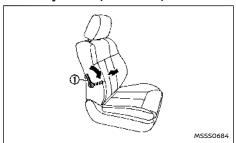
Pull or push the adjusting lever ① to adjust the seat lumbar area until the desired position is achieved.
