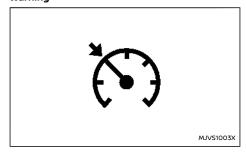
When the system is not operating properly, the chime sounds and the colour of the cruise indicator will change to yellow.
