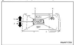
The speed limiter set switches are located on the steering wheel.
