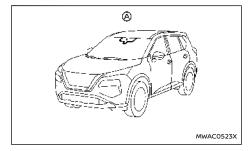
The lane camera unit (A) for the Intelligent Lane Intervention system is located above the inside rearview mirror. To keep the proper operation of the Intelligent Lane Intervention system and prevent a system malfunction, be sure to observe the following:
