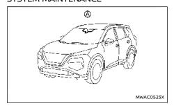
The lane camera unit (A) for the LDW system is located above the inside rearview mirror.
