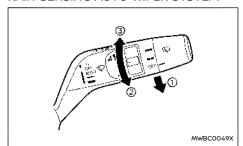
The rain-sensing auto wiper system can automatically turn on the wipers and adjust the wiper speed depending on the rainfall and the vehicle speed by using the rain sensor located on the upper part of the windscreen.
