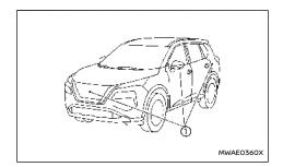
To display the multiple views, the Intelligent Around View Monitor system uses cameras ① located on the front grille, on the vehicle's outside rearview mirrors and one just above the vehicle's rear number plate.
