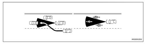
The detection zone of the radar sensor is limited. A vehicle ahead must be in the detection zone for the vehicle-to-vehicle distance detection mode to maintain the selected distance from the vehicle ahead.
