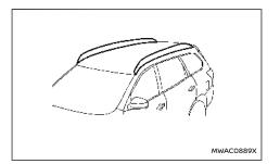
Do not apply any load directly to the roof side rails. Cross bars must be installed before applying load/cargo/luggage to the roof of the vehicle. For additional information, it is recommended that you contact a NISSAN dealer or qualified workshop.
