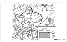
Check the coolant level in the reservoir when the engine is cold. If the coolant level is below the MIN level (2), open the reservoir cap and add coolant up to the MAX level (1).
