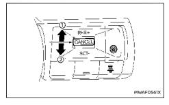
The vehicle set speed can be adjusted.
