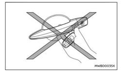
Do not use the lock or capacitive unlock sensors or request switch with the Intelligent Key held in your hand as illustrated. The close distance to the door handle will cause the Intelligent Key system to have difficulty recog-
