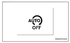
The system can be temporarily deactivated by pressing the Stop/Start OFF switch. Pressing the switch again or restarting the engine by using the ignition switch will reactivate the Stop/Start System.
