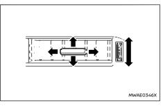
Open/close the vents by moving the control to either direction
