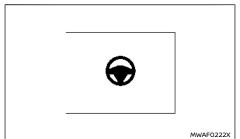
The Steering Assist switch is used to temporarily turn on and off the Steering Assist system.
