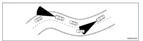
When driving on some roads, such as winding, hilly, curved, narrow roads, or roads which are under construction, the radar sensor may detect vehicles in a different lane, or may temporarily not detect a vehicle travelling ahead. This may cause the Intelligent Forward Collision Warning system to work inappropriately.
