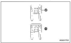
If the fuse is open (a), replace it with a new fuse (a).
