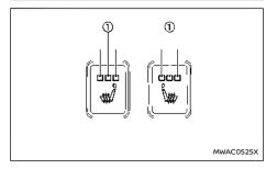
The second row seats are warmed by built-in heaters. The switches are located on the back of the centre console and can be operated independently of each other.
