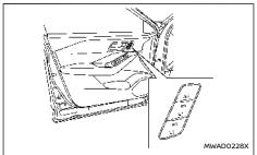
Automatic drive positioner switch (driver's side shown; passenger side similar)
