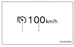
The speed limiter operating condition is shown on the vehicle information display.
