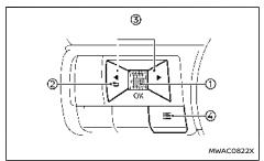
The vehicle information display can be changed using the scroll dial ①, ② ②, and ④ ⑤ ③ located on the steering wheel.
