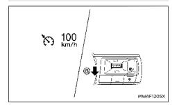
To set cruising speed, accelerate your vehicle to the desired speed, push down the <SET-> (B) switch and release it. (The colour of the cruise indicator changes to green and vehicle set speed indicator comes on.) Take your foot off the accelerator pedal. Your vehicle will maintain the set speed.
