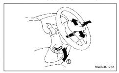
Pull the lock lever  $\Large{\textcircled{1}}$  down and adjust the steering wheel up, down, forward or rearward to the
