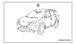
The LDW system will operate when the vehicle is driven at speeds of approximately 60 km/h (37 MPH) and above, and the lane markings are clearly visible on the road.
