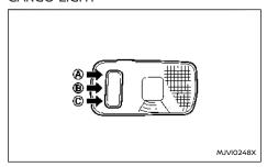
The cargo light has a three-position switch.
