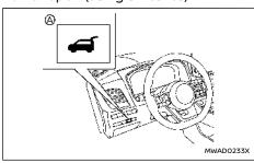
Power back door switch - Instrument panel
