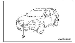
The Intelligent Forward Collision Warning system uses a radar sensor (A) located on the front of the vehicle to measure the distance to a second vehicle ahead in the same lane.
