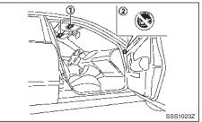
Warning labels about the supplemental air bag system are placed in the vehicle as shown in the illustration.
