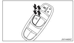
The automatic function is available for the switch that has an  $\overbrace{\mathbf{A}}$  mark on its surface.
