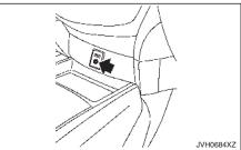
The AUX input jack is located on the lower part of the instrument panel. Compatible audio devices, such as some MP3 players, can be connected to the system through the AUX input jack. Before connecting a device to a jack, turn off the power of the portable device.
