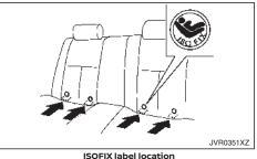
Your vehicle is equipped with special anchor points that are used with ISOFIX child restraint systems.
