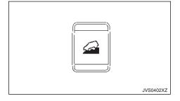
When additional braking is required on steep downhill roads, activate the hill descent control system by pushing the hill descent control switch on.
