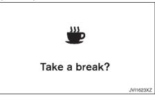
If the system detects that driver attention is decreasing, the message [Take a break?] appears in the vehicle information display and a buzzer sounds when the vehicle is driven at speeds above 60 km/h (37 MPH).
