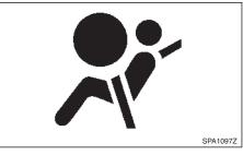
The SRS air bag warning light, displaying 3 in the meter, monitors the circuits for the air bag systems, pre-tensioner seat belt systems and all related wiring.
