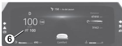
To store the current speed, press the switch **4** (RES/+) or the switch **3** (SET/-): the speed limit replaces the dash-
