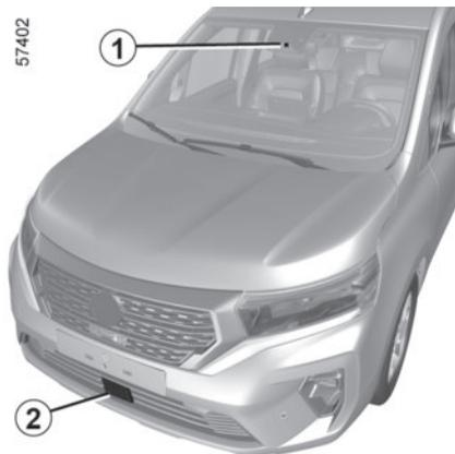
The system uses information from the radar **2** and the camera **1**, to determine the distance between your vehicle:
