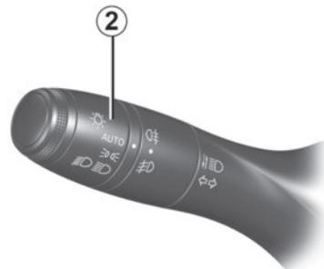
The lights will go out automatically when the engine is switched off, the driver's door is opened or the vehicle is locked. In this case, the next time the engine is started the lights will be switched back on according to the position of the ring **2**.
