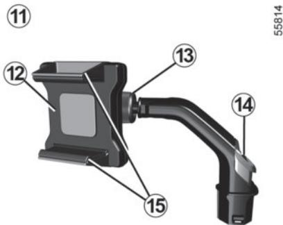
On equipped vehicles, open the storage compartment **A** and insert the phone holder into one of the locations **16** while pressing the button **14**.
