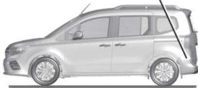
Using information from the radar **2** and the camera **1**, the function triggers corrective action on the vehicle steering system in the event of a risk of collision with a vehicle coming from the opposite direction in the adjacent lane, without the direction indicator having been activated.
