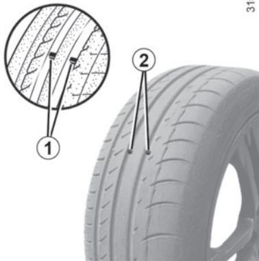
When the tyre tread has been worn to the level of the wear indicators, **these become visible 2**: it is **then** necessary to replace your tyres because the tread rubber is **1.6 mm deep at most, resulting in poor roadholding on wet roads**.
