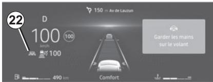
When the "Lane Centring" function no longer detects your hands on the steering wheel, several warning levels will be triggered:
