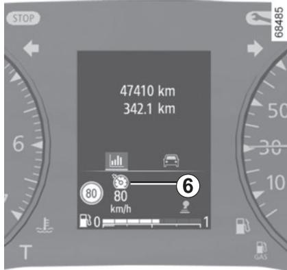
The **6** warning light disappears from the instrument panel to confirm that the function has stopped.
