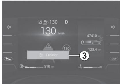
If active emergency braking has caused the vehicle to stop, the vehicle is kept stationary for a short time. Beyond this time limit, the vehicle must be held stationary by the driver keeping their foot on the brake pedal.
