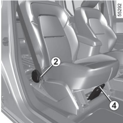
Depending on the seat, raise the lever **2** and tilt the seatback until it reaches the position required.
