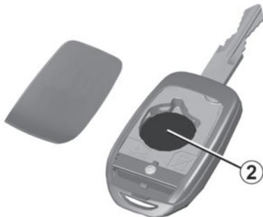
**Note:** it is not advisable to touch the electronic circuit in the key cover when replacing the battery.
