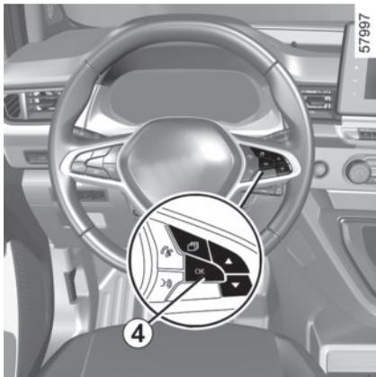
With one of the trip settings selected as the display, press and hold switch **4** "OK" until the display resets to zero.
