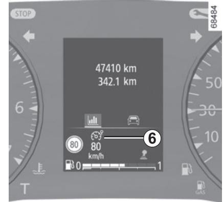
Press the switch **1**. The **6** warning light appears in grey. The "Speed limiter ON" message appears on the instrument panel accompanied by dashes to indicate that the speed limiter function is in operation and waiting to store a limit speed.
