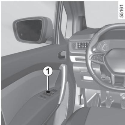
The one-touch mode works in addition to the operation of the electric windows described previously.
