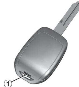
Open the case at slot **1** using a flat-blade screwdriver or similar tool and replace the battery **2** observing the type and polarity shown on the back of the cover.
