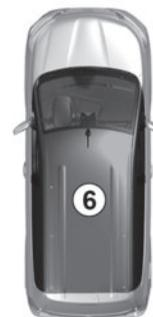
**With the engine running,** if the Intelligent Key is no longer in zone **6** after a door has been opened and closed, the "Keycard Not Detected" message is displayed to warn you that the Intelli-
