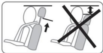
**When the headrest is set at the lowest position, this is for storage only:** it should not be in this position when the seat is occupied.
