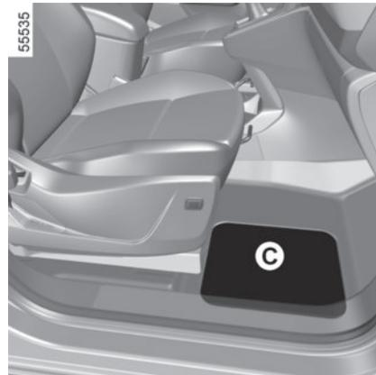
Depending on the vehicle, in the event of a puncture use the kit located in the storage compartment under the flap **C** at the footwell of the front right-hand seat.
