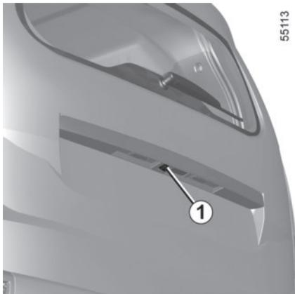
Depending on the vehicle, when the reverse gear is engaged, the camera **1** located on the tailgate or on the rear hinged door transmits a view of the surroundings behind the vehicle to:
