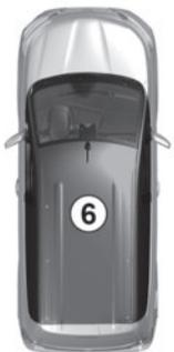
Locking when moving away is not possible if the Intelligent Key is in the zone **6**.
