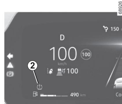
When fitted to the vehicle, this system notifies the driver if one or more tyres lose pressure.
