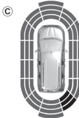
The system is able to detect most obstacles located near the rear and, depending on the equipment, near the front and sides of the vehicle.
