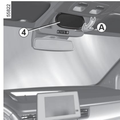
The child minder mirror allows you to keep an eye on your child in the back seat. Pull downwards (movement **A**) to set it to its position of use.
