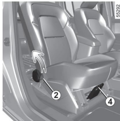
Depending on the vehicle, the seatback on the passenger side may be folded down onto the seat base to create a flat position.
