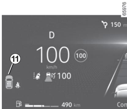
**Driver's seat belt reminder warning light and, depending on the vehicle, front passengers' seat belt reminder warning light**
