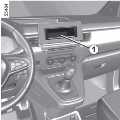
Unclip the blanking cover. The connections (aerial, "+" and "-" supply, speaker wiring) are located behind it.
