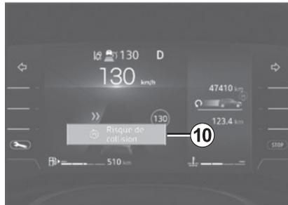
When driving at a speed between approximately 43 mph (70 km/h) and 68 mph (110 km/h), if there is a risk of col-
