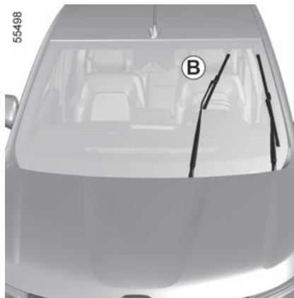
To refit the wiper blade **2**, insert it into its housing in the arm **3**, then clip it until you hear a click. Make sure that the blade is correctly locked in position.
