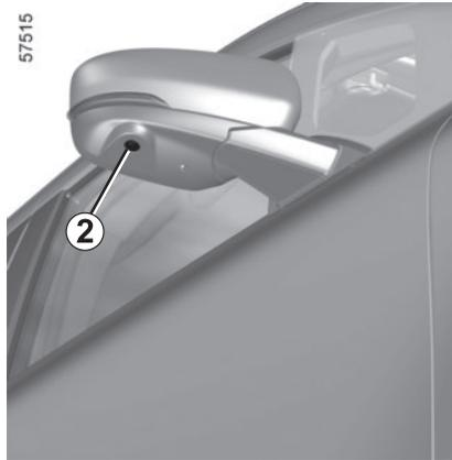
The camera fitted in the door mirror transmits the side view to the multimedia screen **5**.
