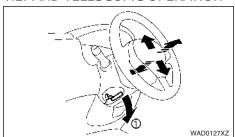
Pull the lock lever 1 down and adjust the steering wheel up, down, forward or rearward to the desired position. Push the lock lever up securely to lock the steering wheel in place.
