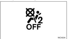
1. If the child restraint is installed on the front passenger seat, switch the power switch ON. The <PASSENGER AIR BAG OFF> 2 light, located on the roof console, should illuminate. If the <PAS-SENGER AIR BAG ON> Ight is illuminated, see "Supplemental Restraint System (SRS)" later in this section.) Move the child restraint to another seating position. Have the system checked by a NISSAN dealer or qualified workshop.
