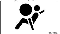
The SRS air bag warning light, displaying the instrument panel, monitors the circuits of the supplemental restraint system. The circuits monitored are:
