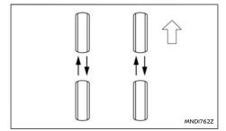
NISSAN recommends that tyres be rotated every 10.000 km (6.000 miles) for Two-Wheel Drive (2WD) vehicles and 5,000 km (3,000 miles) for Four-Wheel Drive (4WD) vehicles.
