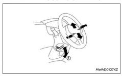
Pull the lock lever 10 down and adjust the steering wheel up, down, forward or rearward to the
