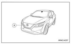
The I-FCW system uses a radar sensor (A) located on the front of the vehicle to measure the distance to a second vehicle ahead in the same lane.
