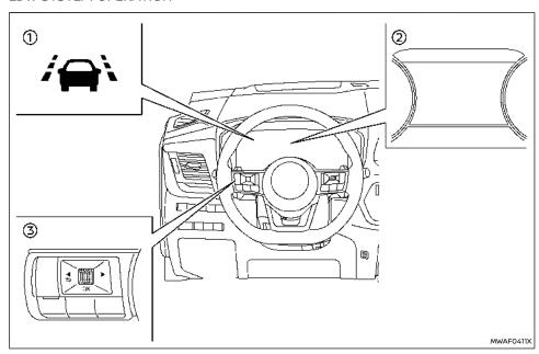
When the vehicle approaches either the left or the right side of the travelling lane, the steering wheel will vibrate, and the LDW indicator on the vehicle information display will blink to alert the driver.
