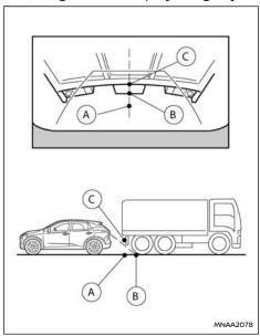
The position © is shown farther than the position ® in the display. However, the position © is actually at the same distance as the position ®. The vehicle may hit the object when reversing to the position ® if the object projects over the actual moving course.
