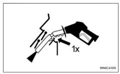
The fuel tank is not equipped with a fuel-filler cap. After opening the fuel-filler lid, insert the fuel pump nozzle directly into the fuel-filler opening and only to the first notch on the bottom of the nozzle When the fuel pump nozzle is pulled out, the fuelfiller opening will be sealed.
