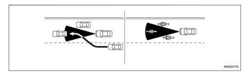
The detection zone of the radar sensor is limited. A vehicle ahead must be in the detection zone for the ICC system to maintain the selected distance from the vehicle ahead. A vehicle ahead may move outside of the detection zone due to its position within the same lane of travel. Motorcycles may not be detected in the same lane ahead.
