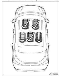
In vehicles fitted with Rear Occupant Detection, in addition to the Seat Belt Warning Light, the Occupant Status Display will be shown in the Vehicle Information Display (See "Vehicle information display" (P.82).) when any vehicle occupant's seat belt is not fastened.
