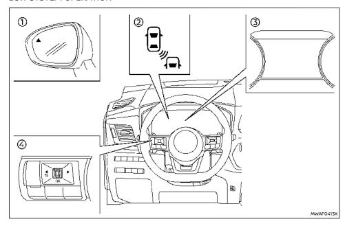
chimes (twice) and the BSW LED indicator light and the BSW indicator will flash. The BSW LED indicator light and the BSW indicator continue to flash until the detected vehicle leaves the detection zone.
