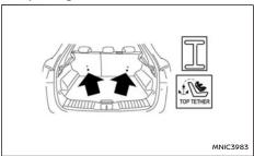
Anchor points are located on the seatback behind the rear outer seating positions and should only be used for child restraints in the rear outer positions.
