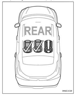
In vehicles not fitted with Rear Occupant Detection, the Rear Passenger Seat Belt Display will be shown in the Vehicle Information Display (See 'Vehicle information display' (P.82)) for approximately 65 seconds when the ignition is switched ON while any rear seat belt is unfastened. The driver can acknowledge the display by pushing the <OK> steering wheel switch.
