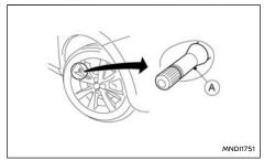
A Tyre valve with sensor
