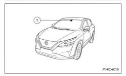
Multi-sensing front camera The Steering Assist system uses a multi-sensing front camera (1) installed behind the windscreen to monitor the lane markers of your travelling lane.
