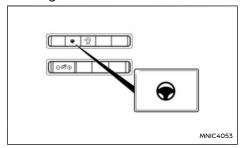
When the system malfunctions, it turns off automatically. The Steering Assist status warning illuminates (yellow) and a warning message is displayed in the vehicle information display. A chime may sound depending on the situation.
