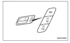
Two positions for the driver's seat and outside mirrors can be stored in the Driving Position Memory System memory. Follow these procedures to use the memory system.
