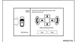
Adjust the target parking rectangle using the arrow keys on the screen so that the clearance guidelines do not overlap any obstacles around the vehicle
