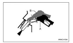
Hold the fuel pump nozzle in position A (shown). Holding the fuel pump nozzle in position B may cause fuel pump nozzle to shut off before the tank is full.
