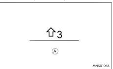
The shift indicator (A) located in the lower part of the vehicle information display can help to improve the level of environmentally friendly driving. Following the shift indicator by changing to the suggested gear when displayed may improve fuel
