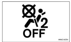
If the child restraint is installed on the front passenger seat, switch the ignition ON. The <PASSENGER AIR BAG OFF> light, located on the roof console, should illuminate. If the <PASSENGER AIR BAG ON> light is illuminated, see "Supplemental Restraint System (SRS)" (P.51). Move the child restraint to another seating position. Have the system checked by a NISSAN dealer or qualified workshop.
