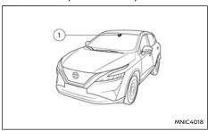
The sensor ① of the rain-sensing auto wiper system located on the upper part of the wind-screen, in front of the rear view mirror, can automatically turn on the wipers and adjust the wiper speed depending on the rainfall intensity and the vehicle speed when the lever in the <AUTO> position.
