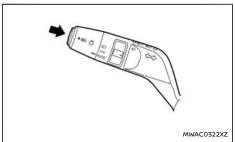
To switch on the Adaptive Driving Beam system. push the switch as illustrated when it is in the AUTO position. The Adaptive Driving Beam indicator light  $\Xi(A)$  in the instrument panel will illuminate.
