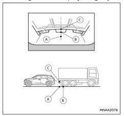
The position © is shown further than the position ® in the display. However, the position © is actually at the same distance as the position ®. The vehicle may hit the object when moving toward the position ® if the object projects over the actual moving course.
