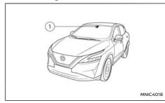
The lane camera unit ① for the ILI system is located above the interior rear view mirror. To maintain the proper operation of the ILI system and prevent a system malfunction, be sure to observe the following:
