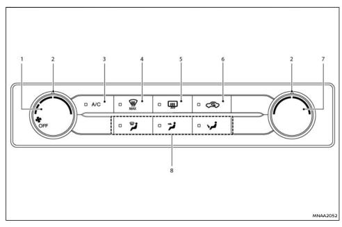
To turn off the heater and air conditioner, turn the fan speed control  $\mbox{\$}$  dial to the OFF (0) position.
