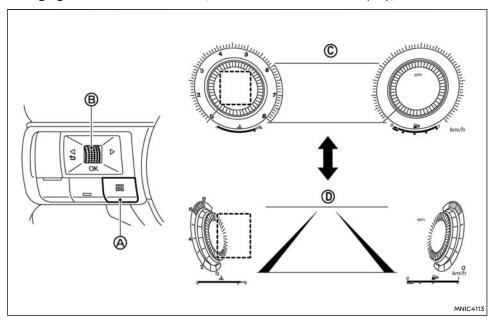
For models with full-screen display, the meter screen view can be changed from Classic View © to Enhanced View (1) to expand the vehicle information display area.
