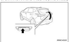
To open the tailgate, unlock it. Pull up the tailgate to open.
