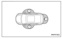
The Intelligent Key functions can only be used when the Intelligent Key is within the specified operating range from the request (lock/unlock) button (1).
