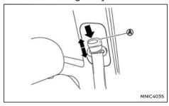
The shoulder belt anchor height should be adjusted to the position that is best for you. (See "Precautions on seat belt usage" (P.27).)
