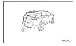
To display the rear view, the Rear-view Monitor system uses a camera ① located just above the vehicle's number plate.
