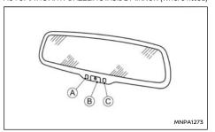
The inside mirror is designed so that it automatically adjusts the reflection according to the intensity of the following vehicle's headlights on the sensor (C)
