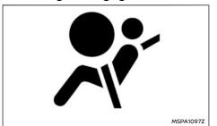
The SRS air bag warning light, displaying 🥻 in the instrument panel, monitors the circuits of the supplemental restraint system. The circuits monitored are:
