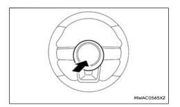
To sound the horn, push the centre pad area of the steering wheel.
