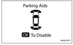
When the vehicle is in R (Reverse) and the [Parking Aids] screen is displayed in the vehicle information display the RAB system can be disabled temporarily by pushing the <OK> switch on the steering wheel.
