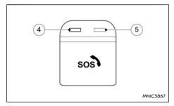
The indicator lights ⓐ and ⑤ above the **<SOS>** button indicate the status of the vehicle emergency call system. If the indicator light is illuminated red or no indicator light is illuminated the emergency call may not connect to the emergency call centre when the **<SOS>** button is pressed. Also an automatic emergency call may not be sent when a collision occurs.
