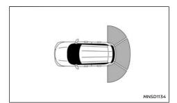
The parking sensor (sonar) system sounds a tone to inform the driver of obstacles near the rear bumper.
