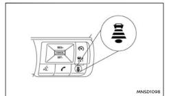
The distance to the vehicle ahead can be selected when the ICC is in standby mode or the ICC is active, depending on the traffic conditions.
