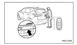
When the Intelligent Key is within the range of operation, the door locks can be locked or unlocked by pushing the door handle request
