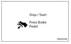
This guidance is displayed when the vehicle is stopped if the Stop/Start System is deactivated due to not fully depressing the brake pedal.
