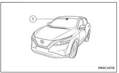
The lane camera unit (1) for the ILI system is located above the interior rear view mirror. To maintain the proper operation of the ILI system and prevent a system malfunction, be sure to observe the following:
