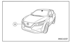
The sensor for the ICC system is located on the front of the vehicle  $\triangle$ .
