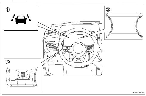
right side of the travelling lane, the steering wheel will vibrate, a warning chime will sound (only when Steering Assist is active) and the LDW indicator on the vehicle information display will blink to alert the driver.
