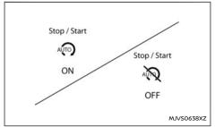
The Stop Start system ON or OFF message is displayed for a few seconds in the vehicle information display when the Stop/Start System OFF switch is pressed.
