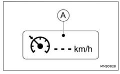
When pushing the Drive Assist switch on, the conventional (fixed speed) cruise control mode display and indicators are displayed in the vehicle information display. After you hold the Drive Assist switch for longer than about 1.5 seconds, the ICC system display goes out. The cruise indicator appears. You can now set your desired cruising speed. Pushing the Drive Assist switch again will turn the system completely off.
