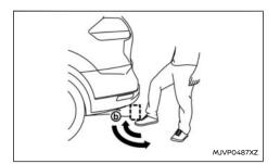
The tailgate can be operated using a guick kicking motion under the centre of the rear bumper.
