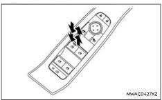
The automatic function enables a window to fully open or close without holding the switch down or up.
