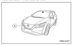
The radar sensor is located on the front of the vehicle (A).
