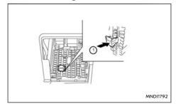
To reduce battery drain, the extended storage fuse switch ① comes from the factory switched off. Prior to delivery of your vehicle, the switch is pushed in (switched on) and should always remain on.
