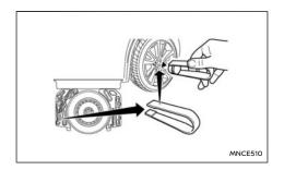
Alloy wheels (where fitted): Alloy wheel bolts have a plastic cap that can be removed using tweezers (where fitted) from the tool kit.
