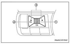
The vehicle information display can be changed using the scroll dial (1), (2), and (3) (3) located on the steering wheel.
