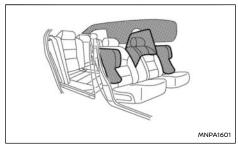
The Supplemental side-impact air bag system consist of two Front Side Air Bags located in the outside of the seatback of the front seats, two Curtain Air Bags located in the roof side trim and dependent on vehicle specification one Front Centre Air Bag (where fitted) located in the inside of the seatback of the driver seat
