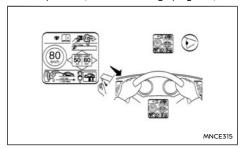
Remove the speed restriction sticker from the compressor, then place it in a location where the driver can see it while driving.
