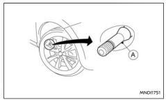
A Tyre valve with sensor
