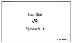
This message is displayed when the Stop/Start System is malfunctioning.
