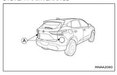
The two radar sensors (A) for the BSW/Intelligent Blind Spot Intervention system are located near the rear bumper.
