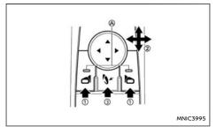
Select the left or right outside rear-view mirror using the appropriate selection switch (1) (the indicator light (A) on the selected mirror switch illuminates), then adjust the mirror to the desired position by pushing the control as illustrated 2.
