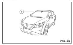
The lane camera unit ① for the Intelligent Lane Intervention system is located above the interior rear view mirror. To maintain the proper operation of the Intelligent Lane Intervention system and prevent a system malfunction, be sure to observe the following:
