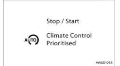
This guidance is displayed when the vehicle is stopped if the Stop/Start System is deactivated due to not fully releasing the clutch pedal.
