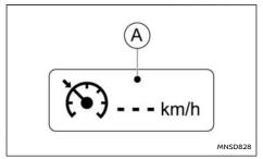
When pushing the ICC ON/OFF switch on, the conventional (fixed speed) cruise control mode display and indicators are displayed in the vehicle information display. After you hold the ICC ON/OFF switch for longer than about 1.5 seconds, the ICC system display goes out. The cruise indicator appears. You can now set your desired cruising speed. Pushing the ICC ON/OFF switch again will turn the system completely off.
