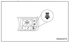
The distance to the vehicle ahead can be selected when the ICC is in standby mode or the ICC is active, depending on the traffic conditions.
