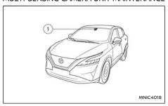
The lane camera unit 1 for the LDW system is located above the interior rear view mirror. To maintain the proper operation of the LDW system and prevent a system malfunction, be sure to observe the following:
