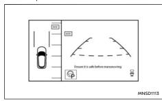
Press Parking Mode button nd check the parallel parking mode is displayed.
