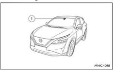
The lane camera unit (1) for the LDW system is located above the interior rear view mirror. To maintain the proper operation of the LDW system and prevent a system malfunction, be sure to observe the following:
