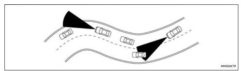
When driving on some roads, such as winding, hilly, curved, narrow roads, or roads which are under construction, the radar sensor may detect vehicles in a different lane, or may temporarily not detect a vehicle travelling ahead. This may cause the radar system to decelerate or accelerate the vehicle.
