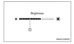
The instrument brightness control switch can be operated when the ignition is ON. When the switch
