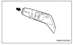
To activate the high beam assist system, push the switch as illustrated when it is in the AUTO position. The high beam assist indicator light  $\Xi(A)$ in the instrument panel will illuminate
