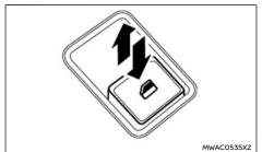
The passenger's switch can control its corresponding window. When the window lock button on the driver's switch is pushed, rear passenger's switches cannot be operated, but the front passenger's switch can still be operated.
