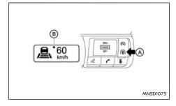
To turn the cruise control on, quickly push and release the Drive Assist switch (a). A pop-up display showing Drive Assist System status will appear. The ICC system **ON** indicator (grey), and set vehicle speed indicator (a) come on.
