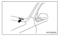
The Vehicle identification number (VIN) is located as shown.
