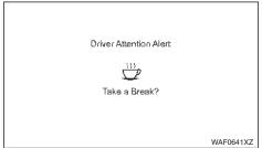
If the system detects that driver fatigue increases or that driver attention is decreasing, the message [Take a break?] appears in the Vehicle Information Display and a chime sounds when the vehicle is driven at speeds above 60 km/h (37 MPH).
