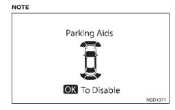
When the transmission is in R (Reverse) and the [Parking Aids] screen is displayed in the vehicle information display the RAB system can be disabled temporarily by pushing the <OK> switch on the steering wheel.
