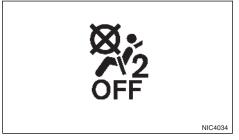
If the child restraint is installed on the front passenger seat, switch the ignition ON. The <PASSENGER AIR BAG OFF> ight, located on the roof console, should illuminate. If the <PASSENGER AIR BAG ON> light is illuminated, see "Supplemental Restraint System (SRS)" later in this section.) Move the child restraint to another seating position. Have the system checked by a NISSAN dealer or qualified workshop.
