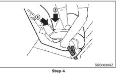
4. Remove any additional slack from the seat belt; press downward ③ and rearward ④ firmly in the centre of the child restraint with your hand to compress the vehicle seat cushion and seatback while pulling up on the seat belt.
