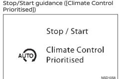
This guidance is displayed when the vehicle is stopped if the Stop/Start System is deactivated because the air conditioner (cooling, heating or dehumidifying functions) is given priority.
