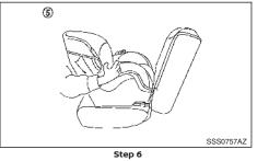
Test the child restraint before you place the child in it (5). Push the child restraint from side to side and tug it forward to make sure that it is held securely in place.  Check to make sure that the child restraint is properly secured prior to each use. If the child restraint is loose, repeat steps 3 through 6.
