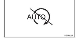
This indicator is displayed when the vehicle is stopped if the engine is prevented from automatically stopping by the Stop/Start System due to inhibition conditions.
