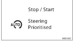
This guidance is displayed when the vehicle is stopped if the Stop/Start System is deactivated due to steering operation being detected.
