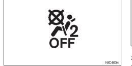
If the child restraint is installed on the front passenger seat, switch the ignition ON. The <PASSENGER AIR BAG OFF> ign light, located on the roof console, should illuminate. If the <PASSENGER AIR BAG ON> light is illuminated, see "Supplemental Restraint System (SRS)" later in this section.) Move the child restraint to another seating position. Have the system checked by a NISSAN dealer or qualified workshop.
