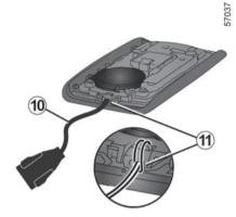
Insert the hand strap into the component *11* and pass the end of the strap through the buckle.
