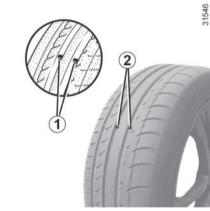
The tyres must be in good condition and the treads must have sufficient depth: tyres approved by our Technical Department have wear warning strips **1** which are **indicators moulded into the tread at several points**. When the tyre tread has been worn to the level of the wear indicators, **they become visible 2**: it is then necessary to replace your tyres because the tread rubber is 1.6 mm deep at most, resulting in poor road-holding on wet roads.
