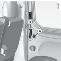
Pull the lever **3** towards the rear and open the sliding door until it locks into position.
