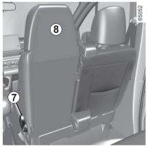
The front centre seat is equipped with a folding seatback 8 to enable an emergency exit.
