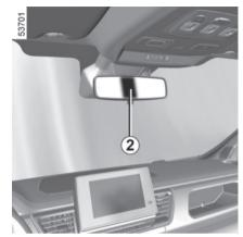
Note: make sure that the reversing camera is not obscured (by dirt, mud, snow, condensation, etc.).
