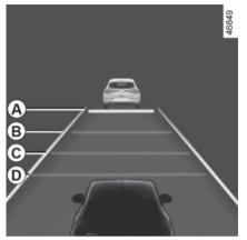
You can vary the safe distance from the vehicle in front at any time by pressing switch *2* repeatedly.
