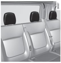
Insert the headrest rods into the holes (tilt the seatback if necessary). Lower the headrest as far as it will go, then lift until it locks into place. Check that each rod *2* is locked on the seatback.
