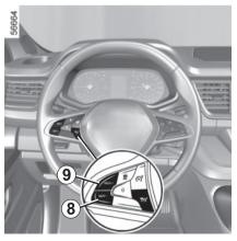
To adapt the speed limiter, cruise control or adaptive cruise control setpoint to detected speed limits, press switch 8 (SET/-) or 9 (RES/+).
