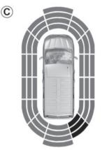
The system is able to detect most objects located near the rear and, depending on the equipment, near the front and sides of the vehicle
