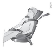
From 15 kg or 4 years, the child can travel using a booster seat which will enable the seat belt to be adapted to suit the size and shape. The booster seat cushion must be fitted with guides to position the seat belt on the child's thighs rather than the stomach. It is recommended that you use a seatback which can be adjusted in terms of height to position the seat belt in the centre of the shoulder. It must never rest on the neck or on the arm.
