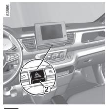
Press the switch *2*. This switch activates all four direction indicators and the side indicator lights simultaneously. It must only be used in an emergency to warn drivers of other vehicles that you have had to stop in an area where stopping is prohibited or unexpected, or that you are obliged to drive under special conditions.
