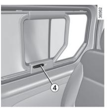
Move the handle 4 and slide the window to the desired notch.
