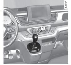
Shift the selector lever 1 to D position, then shift the lever to the right to M position.
