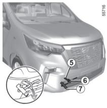
Unclip the cover *5* by inserting a flatblade screwdriver or similar under the cover.
