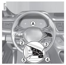
Press the switch *2* as many times as required to reach the "Vehicle" tab.
