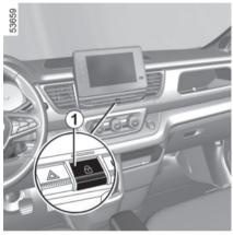
When the ignition is on, the indicator light integrated in switch 1 informs you of the locking status of the opening elements:
