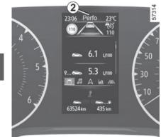
Each time the engine is switched off, performance mode will be deactivated and it will be necessary to select it again.
