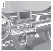
Socket **1** and, depending on the vehicle, sockets **2**, **3** and **4** are designed for connecting accessories which have been approved by our Technical Department and with a power not exceeding 120 Watts (12 V).
