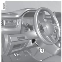
Pull the lever 1 and set the steering wheel to the required position, then push the lever beyond the point of resistance to lock the steering wheel in place.
