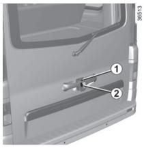
The tailgate is locked and unlocked by pressing the remote control button.
