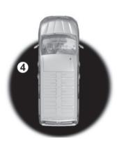
With the card on you and the doors and luggage compartment door closed, move away from the vehicle: it will be locked automatically as soon as you leave the access zone *4*.
