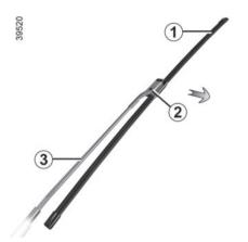
Lift the windscreen wiper arm **3**, press the button **2** to release the blade **1**.
