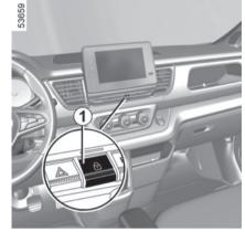
The switch 1 controls all the doors simultaneously.
