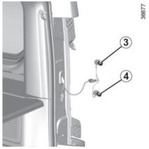
**Direction indicator lights** *3* Pear-shaped, bayonet type bulb PY 21W.
