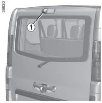
When shifting to reverse gear, the camera 1 located on the tailgate or, depending on the vehicle, on the rear hinged door, transmits a view of the area behind the vehicle to the rear view mirror 2 or, depending on the vehicle, to the multimedia display 3 accompanied by two moving or fixed guide lines 4 and 5.
