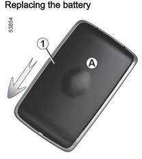
When the "Keycard Battery Low" message appears on the instrument panel, replace the card battery:
