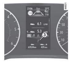
Depending on the vehicle, to obtain optimum consumption levels, a warning light on the instrument panel lets you know the best time to move up or down a gear:
