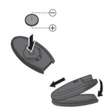
When refitting, proceed in the reverse order, then press one of the buttons on the Intelligent Key four times while standing near the vehicle: the next time the vehicle is started, the message will disappear.
