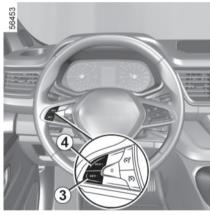
The limit speed may be changed by pressing repeatedly or holding down:
