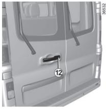
If one of the rear opening elements is open, press button **9**, **10** or **12** to lock the front doors.
