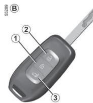
Using remote control **A** or **B**, press button **3** to unlock the sliding side doors and the rear hinged doors or the tailgate. (j) Remote controls A or Bvan version
