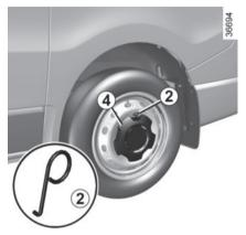
Remove it using the hubcap tool 2 (located in the tool kit) by engaging the hook in the opening near the edge of the trim.
