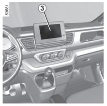
With the engine running, from the multimedia screen *3* you can add or remove the guide lines and adjust the camera image settings (brightness, contrast, etc.). Please refer to the multimedia instructions for further information.
