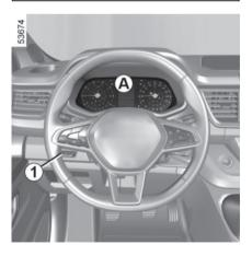
Instrument panel A: lights up when the ignition is switched on. Press or raise the switch 1 as many times as required to adjust the intensity.
