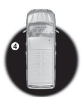
With the Intelligent Key on you and the doors and luggage compartment closed, move away from the vehicle: it will lock automatically once you have left the access zone 4.
