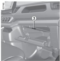
Remove the lens using a tool such as a flat-blade screwdriver.
