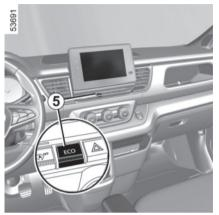
ECO mode is a function which optimises fuel consumption. It affects certain driving operations (acceleration, shifting gears, cruise control, deceleration, etc.).
