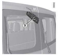
Remove the light sideways from the outside to access the bulb **9**.
