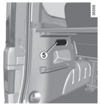
Remove the lens using a tool such as a flat-blade screwdriver.
