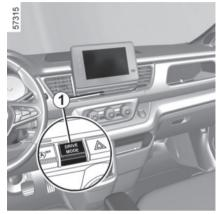
Press button **1** until the "Perfo" message is displayed in zone **2** on the instrument panel to confirm the activation.
