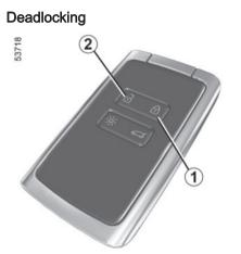
If the vehicle is equipped with a deadlocking function, this allows you to lock the opening elements and to prevent the doors from being unlocked using the interior handles (for example, by breaking the window and then trying to open the door from the inside).
