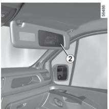
(depending on the vehicle) Lower the sun visor to access the wide-angle rear view mirror.
