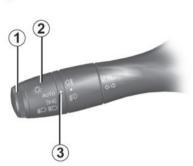
Turn the ring 2 until the AUTO symbol is opposite the mark 3: with the engine on, the dipped beam headlights switch on or off automatically according to the exterior light level, without any action on the stalk 1.
