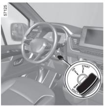
Turn the ignition key to the "ON" position 2 and hold this position until the
