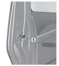
With the door open, turn the screw **5** (using the end of the key) and close the door.
