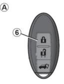
After approximately 15 minutes with the Intelligent Key in the detection zone 4, locking when moving away from the vehicle is deactivated. To lock the vehicle, press button 6 on the Intelligent Key or, depending on the vehicle, button 2 on the handle 1.
