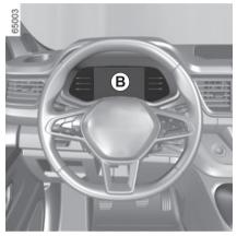
Instrument panel B: lights up when the janition is switched on. Press or raise the switch 1 as many times as required to adjust the intensity.
