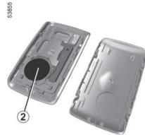
To refit, proceed in the reverse order then press one of the buttons on the card four times while you are near the vehicle: the next time the vehicle is started, the message will disappear.
