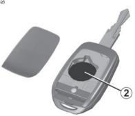
When refitting, ensure that the cover is correctly clipped on and the screw tightened.
