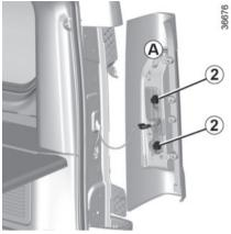
Turn the lights unit slightly and release it to access the bulb holder *2*.
