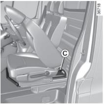
Depending on the vehicle, in the event of a puncture, use the kit located in the tool kit underneath the driver's seat.
