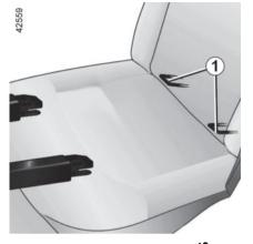
The two rings **1**, identified by a wark, are located between the seatback and the seat base
