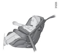
Up to 18 kg or 4 years, the child may travel on a forward-facing seat. Choose your seat according the child's size: their head and abdomen are the areas which must be most protected. A forward-facing child seat which is firmly attached to the vehicle will reduce the risk of impact to the head. Ensure your child travels in a forward-facing seat with a harness or buckle for as long as their size permits.
