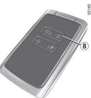
If the card has been within the access zone *3* for longer than approximately 15 minutes, the "locking when moving away" function is deactivated. To lock the vehicle, press the button *8* on the card.
