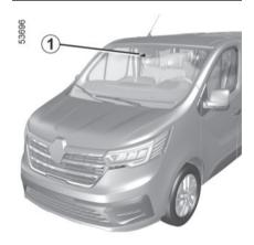
Using information from the camera 1, the function warns the driver if the vehicle crosses a line (continuous or broken) without having activated the direction indicator lights.
