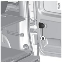
For each door, pull the handle  $\boldsymbol{6}$  to release the door check strap  $\boldsymbol{7}$ . Open the door as far as possible.
