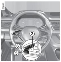
You can vary the speed by repeatedly pressing (small increments) or pressing and holding (large increments) switch *5* or *6*:
