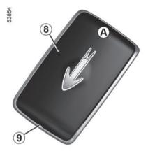
Slide the rear casing **8** downwards while pressing on area **A**.
