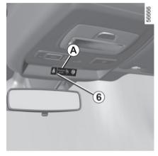
This warning light appears on the central display **A** when the vehicle ignition is switched on and if the driver's and/or front passenger's seat belt(s) (if the passenger seat is occupied) is not fastened.
