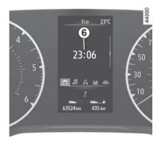
Set the hour using control 3 or 4, then press the switch 5 "OK" to confirm.
