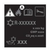
The refrigerant fluid circuit (of which some components are hermetically sealed) may contain fluorinated greenhouse gases.
