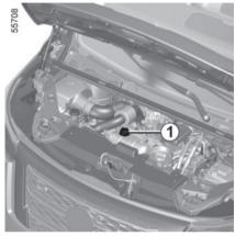
With the ignition switched off and the vehicle parked on flat ground, the level when cold must be between the "MI-NI" and "MAXI" marks indicated on the coolant reservoir 1.
