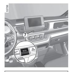
On vehicles equipped with ECO mode (switch 7): when activated, ECO mode can reduce the performance of the heating and/or air conditioning → 213.
