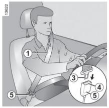
Unwind the belt **slowly and smoothly** and ensure that the buckle **3** locks into the catch **5** (check that it is locked by pulling on the buckle **3**).
