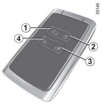
**1.** Unlocking the front doors and, depending on the vehicle, the sliding side door in Secure mode, or unlocking all the opening elements in Access mode.
