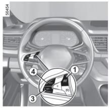
When a limit speed has been set but not yet reached, driving is similar to driving a vehicle without the speed limiter function.
