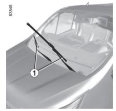
With the ignition on and the ignition switched off, lower the windscreen wiper stalk fully: the wipers stop in a position away from the bonnet.
