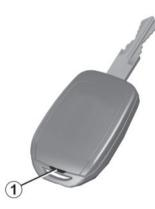
Open the case at slot **1** using a flatblade screwdriver or similar tool and replace the battery *2* observing the type and polarity shown on the back of the cover.
