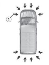
Ultrasonic sensors, indicated by arrows *1*, are fitted in the bumpers to detect obstacles near the vehicle.
