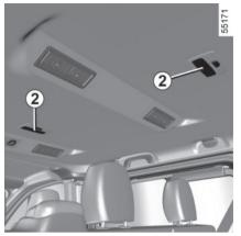
**Bulb type 2:** W5W (depending on the vehicle) Replace the bulb and refit the lens.
