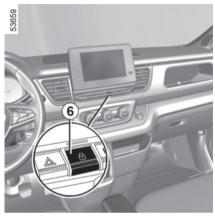
The switch  $\boldsymbol{\theta}$  simultaneously controls the doors and the luggage compartment door.
