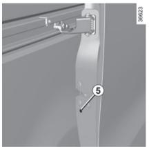
To make it impossible for the rear doors to be opened from the inside: on each door, pivot the bolt **5** and close the door.
