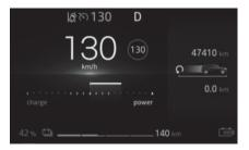
Press switch **1** until the warning light is displayed in green on the instrument panel. The "Cruise control ON" message appears on the instrument panel accompanied by dashes to indicate that the cruise control function is in operation and waiting to store a cruising speed.
