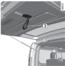
Lower the tailgate, initially using the interior handle **3**.
