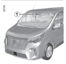
Using the information from the camera 1, this function informs the driver of the time interval between their vehicle and the vehicle in front so that a safe
