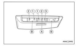
The room light (A) has a three-position switch. When the switch is in the on position 3, the light illuminates
