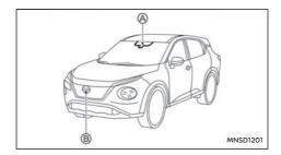
(A) located above the inside mirror to monitors the lane markers on the travelling lane and to detect other vehicles.
