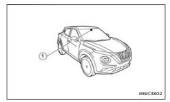
The sensor (1) of the rain-sensing auto wiper system located on the upper part of the windscreen, in front of the rear view mirror, can automatically turn on the wipers and adjust the wiper speed depending on the rainfall intensity and the vehicle speed when the lever in the <AUTO> position.
