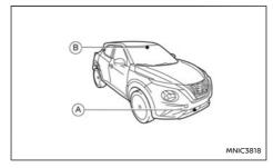
The IEB system uses a radar sensor (A) located at the front of the vehicle and a camera installed behind the windscreen (B) to measure the distance to the vehicle ahead in the travelling lane.
