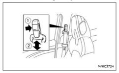
The shoulder belt anchor height should be adjusted to the position that is best for you. (See "Precautions on seat belt usage" (P.36).)
