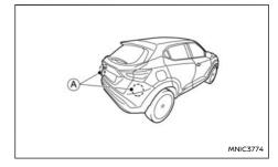
The two radar sensors (A) for the RCTA systems are located near the rear bumper. Always keep the area near the radar sensors clean.
