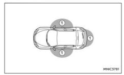
The Intelligent Key functions can only be used when the Intelligent Key is within the specified operating range from the request (lock/unlock) button (1).
