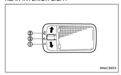
The light switch has three positions: <ON> , <DOOR> and <OFF>.
