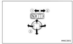
Slide the control to the left ① or to the right ② to select the left or right outside rear-view mirror, then adjust the mirror to the desired position by pushing the control as illustrated ③.
