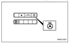
Push the heated steering wheel switch to warm the steering wheel after the hybrid system starts.
