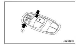
The driver's switch, which is the main switch, can control all of the windows.
