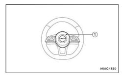
To sound the horn, push the centre pad area (1) of the steering wheel.
