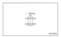
Accordingly, when the TPMS indicator light illuminates, safely stop the vehicle to check the tyres as soon as possible and inflate the tyres to the proper pressure. Driving on a significantly under-inflated tyre causes the tyre to overheat and can lead to tyre failure. Under-inflation also reduces fuel efficiency and tyre tread life which may affect the vehicle's handling and stopping ability.
