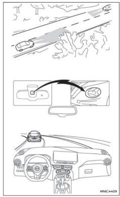
A camera-controlled high beam assistant which changes from low beam to high beam automatically.
