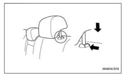
To lower, push and hold the lock knob and push the head restraint down as shown.
