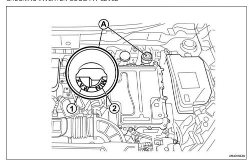
Check the coolant level in the reservoir (A) when the engine and inverter are cold. If the coolant level is below MIN level 2, add coolant up to the MAX level (1).
