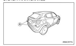
The two radar sensors (A) for the BSW/Intelligent Blind Spot Intervention system are located near the rear bumper.
