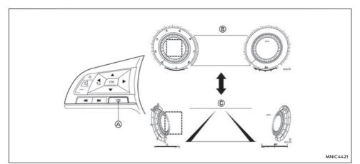
For models with full-screen display, the meter screen view can be changed from Classic View to Enhanced View to expand the vehicle information display area.
