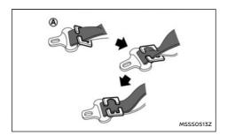
4. Route the seat belt tongue through the child restraint system and insert it into the buckle until you hear and feel the latch engage.
