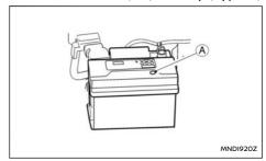
For a maintenance free (MF) battery it is not required to check the fluid level. However, NISSAN recommends to visually check the green indicator A status periodically. If it is not visible, replace the battery as soon as possible.
