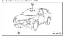
The camera (A) is located on the upper side of the windshield. To keep the Lane Assist system operating properly, be sure to observe the followina:
