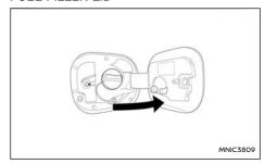
To open the fuel filler lid, push the rear part of the lid inwards, it will then release the latch and open. To lock, close the fuel filler lid securely.
