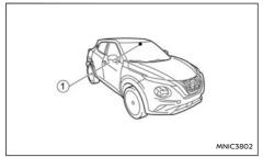
The lane camera unit 1 for the Intelligent Blind Spot Intervention system is located above the interior rear view mirror. To maintain the proper operation of the Intelligent Blind Spot Intervention system and prevent a system malfunction, be sure to observe the following:
