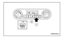
The rear window defogger switch will only operate when the engine is running.
