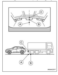
The position © is shown further than the position (B) in the display. However, the position (C) is actually at the same distance as the position (A). The vehicle may hit the object when moving toward the position (A) if the object projects over the actual moving course.
