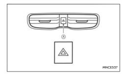
The hazard warning flasher switch operates regardless of the ignition position except when the battery is discharged.
