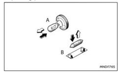
All other lights are either type A, B. When replacing a bulb, first remove the lens and/or cover.
