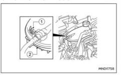
Check the coolant level in the reservoir when the engine is cold. If the coolant level is below MIN level ①, add coolant up to the MAX level ①. If the reservoir is empty, check the coolant level in the radiator when the engine is cold. If there is insufficient coolant in the radiator, fill the radiator with coolant up to the filler opening and also add it to the reservoir up to the MAX level (1).
