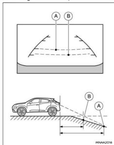
When reversing the vehicle down a hill, the distance guide lines and the vehicle width guide lines are shown further than the actual distance. For example, the display shows 1 m (3 ft) to the place (A), but the actual 1 m (3 ft) distance on the hill is the place (B). Note that any object on the hill is viewed in the monitor closer than it appears.
