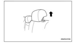
To raise the head restraint, pull it up as shown.
