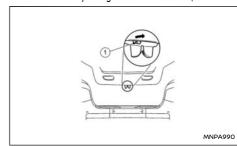
The vehicle's tailgate can be unlocked from the inside when the battery is dead. Tilt the seatback down. Slide the release lever (1) as illustrated. See "Rear seats" (P.33) for more information regarding the seat operation.
