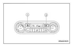
The seats can be warmed by built-in heaters. The switches (1) and (2) located on the heater and air conditioning unit can be operated independently of each other.
