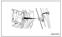
When folding the rear seat forward, the outer seat belts can be stored out of the way using the storage holder shown in the illustration.
