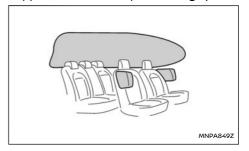
The supplemental side air bags are located in the outside of the seatback of the front seats.
