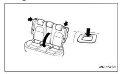
The luggage compartment loading capacity can be increased by folding the rear seats forward as shown
