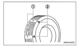
Tyres should be periodically inspected for wear. cracking, bulging or objects caught in the tread. If excessive wear, cracks, bulging or deep cuts are found, the tyre should be replaced.
