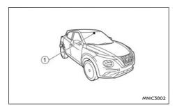
The Traffic Sign Assist (TSA) system provides the driver with information about the most recently detected speed limit. The system captures the road sign information with the multi-sensing front camera unit ① located on the windshield in front of the interior rear-view mirror and displays the detected signs in the Vehicle Information Display.
