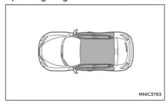
The Intelligent Key can only be used for starting the hybrid system when the Intelligent Key is within the specified operating range (1) as illustrated.
