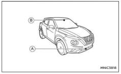
The IEB system uses a radar sensor (A) to measure the distance to the vehicle ahead in the same lane. For pedestrians and cyclists, the IEB system uses a camera (B) installed behind the windscreen in addition to the radar sensor.
