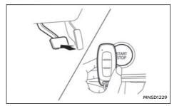
If the battery of the Intelligent Key is discharged, or environmental conditions interfere with the Intelligent Key operation, start the hybrid system according to the following procedure:
