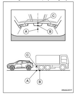
The position © is shown further than the position ® in the display. However, the position © is actually at the same distance as the position ®. The vehicle may hit the object when moving toward the position ® if the object projects over the actual moving course.
