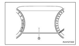
The Vehicle Information Display (1) is located between the power gauge and the speedometer, and it displays warnings and information.
