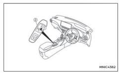
1. With the ignition switch in the ON position, push the automatic brake hold switch (1). The indicator light on the automatic brake hold switch (2) illuminates.
