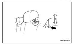
1. Align the head restraint stalks with the holes in the seat. Make sure that the head restraint is facing the correct direction. The stalk with the adjustment notch must be installed in the hole with the lock knob.
