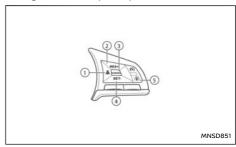
Each time the ICC system is turned on using the blue ProPILOT Assist switch (5), the distance setting reverts to Long.
