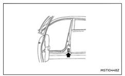
The cold tyre pressure is shown on the tyre placard fixed to the side of the driver's side centre pillar.
