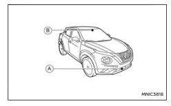
The sensor (A) is located behind the front bumper. The camera (B) is located on the upper side of the windscreen.
