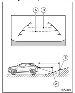
When reversing a vehicle up a hill, the distance guide lines and the vehicle width guide lines are shown closer than the actual distance. For example, the display shows 1 m (3 ft) to the place (A), but the actual 1 m (3 ft) distance on the hill is the place B. Note that any object on the hill is viewed in the monitor further than it appears.
