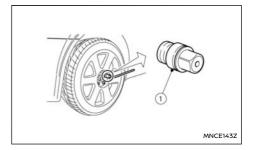
Loosen each wheel bolt by one or two turns anticlockwise with the wheel wrench.
