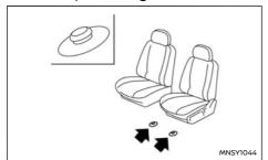
Note that the above illustration is for LHD models This vehicle includes front floor mat brackets (A) to act as a floor mat positioning aid. NISSAN floor mats have been specially designed for your vehicle.
