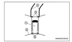
The bird's-eye view shows the overhead view of the vehicle which helps confirm the vehicle position and the predictive course to a parking space.
