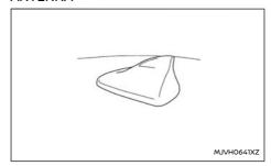
There is a radio antenna on the rear part of the vehicle roof
