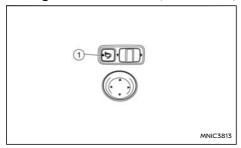
The outside rear-view mirrors fold when the outside rear-view mirror folding button ① is pressed. To unfold, push the button again.
