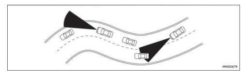
When driving on some roads, such as winding, hilly, curved, narrow roads, or roads which are under construction, the sensor may detect vehicles in a different lane, or may temporarily not detect a vehicle travelling ahead. This may cause the system to work inappropriately.
