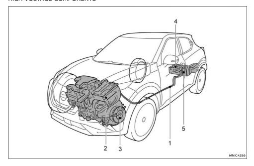
The hybrid system consists of the following high voltage parts.
