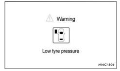
If you now press the **<OK>** switch on the steering wheel, a further screen is displayed to tell you the tyre pressure of all four tyres.
