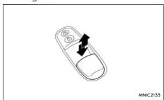
The passenger's switch can control its corresponding window.
