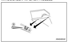
If you wax the surface of the engine bonnet, be careful not to let wax get into the washer nozzle (A). This may cause clogging or improper windscreen washer operation. If wax gets into the nozzle, remove it with a needle or small pin (B).
