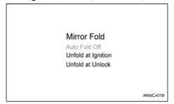
The outside rear-view mirrors automatically unfold when the ignition is switched on or when the vehicle doors are unlocked. Use the [Mirror Fold] menu of the Vehicle Information Display to select the moment that the mirrors are to be automatically folded and unfolded. The Auto fold feature can also be switched off. See "[Vehicle Settings]" (P.89).
