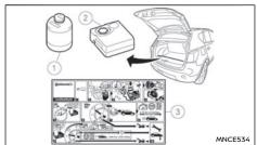
Take the emergency tyre puncture repair kit out of the boot. The repair kit consists of the following items:
