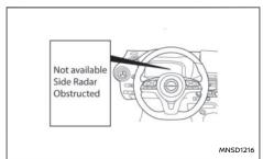
When radar blockage is detected, the system will be deactivated automatically. The [Not available Side Radar Obstructed] warning message will appear in the Vehicle Information Display.
