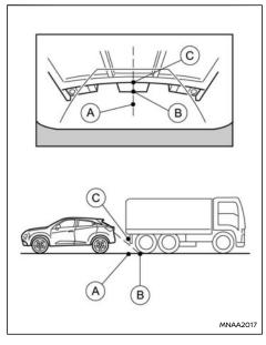
The position  $\bigcirc$  is shown further than the position  $\bigcirc$  in the display. However, the position  $\bigcirc$  is actually at the same distance as the position  $\bigcirc$ . The vehicle may hit the object when moving toward the position  $\bigcirc$  if the object projects over the actual moving course.
