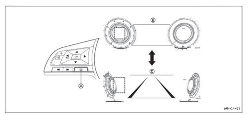
For models with full-screen display, the meter screen view can be changed from Classic View to Enhanced View to expand the vehicle information display area.
