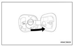
To open the fuel filler lid, push the rear part of the lid inwards, it will then release the latch and open. To lock, close the fuel filler lid securely.
