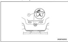
The vehicle's tailgate can be unlocked from the inside when the battery is dead. Tilt the seatback down. Slide the release lever (1) as illustrated. See "Rear seats" (P.33) for more information regarding the seat operation.
