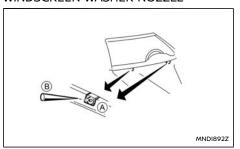
If you wax the surface of the engine bonnet, be careful not to let wax get into the washer nozzle (A). This may cause clogging or improper windscreen washer operation. If wax gets into the nozzle, remove it with a needle or small pin (B).
