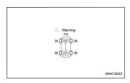
Accordingly, when the TPMS indicator light illuminates, safely stop the vehicle to check the tyres as soon as possible and inflate the tyres to the proper pressure. Driving on a significantly under-inflated tyre causes the tyre to overheat and can lead to tyre failure. Under-inflation also reduces fuel efficiency and tyre tread life which may affect the vehicle's handling and stopping ability.
