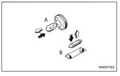
All other lights are either type A, B. When replacing a bulb, first remove the lens and/or cover.
