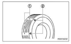
Tyres should be periodically inspected for wear, cracking, bulging or objects caught in the tread. If excessive wear, cracks, bulging or deep cuts are found, the tyre should be replaced.
