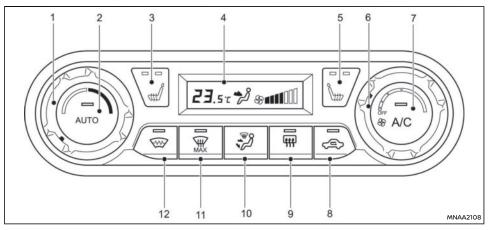
Type B (with seat heater and Thermaclear heated windscreen)
