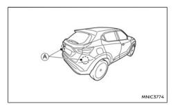
The RCTA system uses radar sensors (A) installed on both sides near the rear bumper to detect an approaching vehicle.
