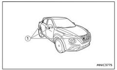
To display the multiple views, the IAVM system uses cameras ① located in the front grille, on the vehicle's outside mirrors and one just above the vehicle's number plate. Do not put anything on the cameras.
