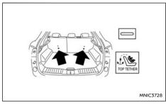
Anchor points are located on the seatback behind the rear outer seating positions and should only be used for child restraints in the rear outer positions.
