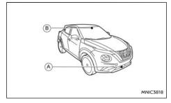
The IEB system uses a radar sensor (a) to measure the distance to the vehicle ahead in the same lane. For pedestrians and cyclists, the IEB system uses a camera (a) installed behind the windscreen in addition to the radar sensor.
