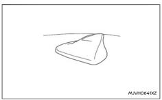
There is a radio antenna on the rear part of the vehicle roof.
