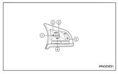
Each time the ICC system is turned on using the blue ProPILOT Assist switch (5), the distance setting reverts to Lona.
