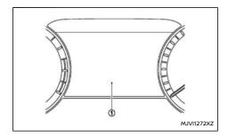
The Vehicle Information Display ① is located between the power gauge and the speedometer, and it displays warnings and information.
