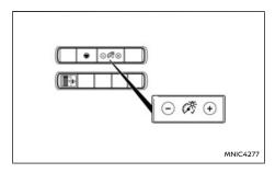
The instrument brightness control switch can be operated when the ignition is in the  ${\bf ON}$  position. When the switch is operated, the brightness adjustment mode appears at the bottom of the vehicle information display.
