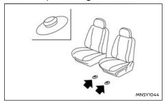
Note that the above illustration is for LHD models This vehicle includes front floor mat brackets (A) to act as a floor mat positioning aid. NISSAN floor mats have been specially designed for your vehicle. Position the mat by placing the floor mat bracket hook into the floor mat grommet hole until the mat clips into position on the hooks while centring
