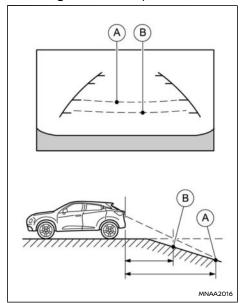
When reversing the vehicle down a hill, the distance guide lines and the vehicle width guide lines are shown further than the actual distance. For example, the display shows 1 m (3 ft) to the place (a), but the actual 1 m (3 ft) distance on the hill
