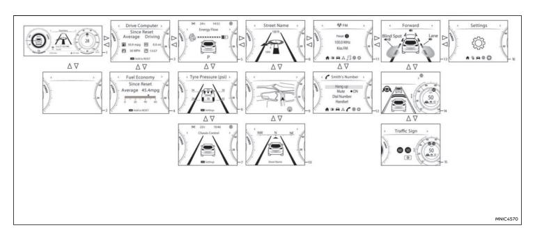
When the ignition is switched ON, the vehicle information display may display the following screens if the vehicle is equipped with them:
