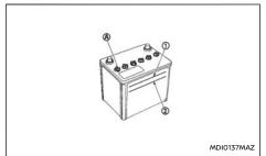
Check the fluid level in each cell. It should be between the UPPER (1) and LOWER (2) level lines.
