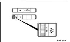
Depending on the number of occupants in the vehicle and the load it is carrying, the headlight axis may be higher than desired. If the vehicle is travelling on a hilly road, the headlights may directly hit the rear-view mirror of the vehicle ahead or the windscreen of an oncoming vehicle. The light axis can be lowered using the switch located on the driver's side of the instrument panel, next to the steering wheel.
