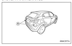
The two radar sensors (A) for the RCTA systems are located near the rear bumper. Always keep the area near the radar sensors clean.
