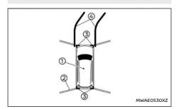
The bird's-eye view shows the overhead view of the vehicle which helps confirm the vehicle position and the predictive course to a parking space.
