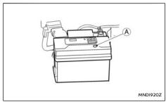
For a maintenance free battery it is not required to check the fluid level. However, NISSAN recommends to visually check the green indicator (A) status periodically. If it is not visible, replace the battery as soon as possible.
