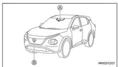
The camera (A) is located on the upper side of the windshield. To keep the Lane Assist system operating properly, be sure to observe the following:
