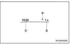
The clock ① and outside air temperature ② are displayed on the upper side of the Vehicle Information Display.
