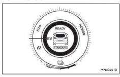
This gauge indicates the actual power consumption and the charging power to the Li-ion battery. For additional information, See "POWER GAUGE" (P.70).
