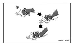
Route the seat belt tongue through the child restraint system and insert it into the buckle until you hear and feel the latch engage.
