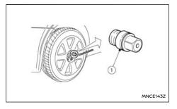
Loosen each wheel bolt by one or two turns anticlockwise with the wheel wrench.
