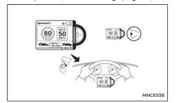
Remove the speed restriction sticker from the compressor, then place it in a location where the driver can see it while driving.
