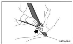
To unfasten the seat belt, push the button on the buckle. The seat belt automatically retracts.
