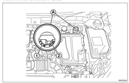
Check the coolant level in the reservoir (A) when the engine and inverter are cold. If the coolant level is below MIN level 2, add coolant up to the MAX level (1).
