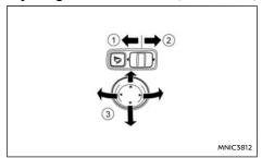
Slide the control to the left (1) or to the right (2) to select the left or right outside rear-view mirror. then adjust the mirror to the desired position by pushing the control as illustrated 3.
