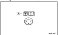
The outside rear-view mirrors fold when the outside rear-view mirror folding button (1) is pressed. To unfold, push the button again.
