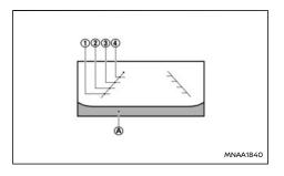
Guiding lines, which indicate the vehicle width and distances to objects with reference to the vehicle body line (a), are displayed on the monitor.
