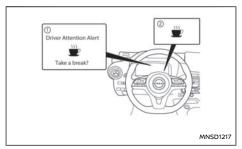
The Intelligent Driver Alertness indicator illuminates in white when a warning is issued and in yellow when a malfunction occurs (where fitted).
