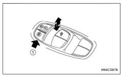
The driver's switch, which is the main switch, can control all of the windows.
