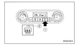
The rear window defogger switch will only operate when the engine is running.
