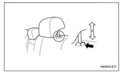
Align the head restraint stalks with the holes in the seat. Make sure that the head restraint is facing the correct direction. The stalk with the adjustment notch must be installed in the hole with the lock knob.
