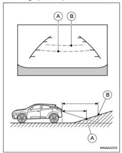
When reversing a vehicle up a hill, the distance guide lines and the vehicle width guide lines are shown closer than the actual distance. For example, the display shows 1 m (3 ft) to the place (A), but the actual 1 m (3 ft) distance on the hill is the place (B). Note that any object on the hill is viewed in the monitor further than it appears.
