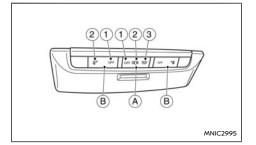
The room light (A) has a three-position switch. When the switch is in the on position 3, the light illuminates
