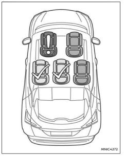
In addition to the Seat Belt Warning Light, the Occupant Status Display will be shown in the Vehicle Information Display (See "Vehicle information display" (P.82)) when any vehicle occupant's seat belt is not fastened.
