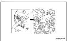
Check the coolant level in the reservoir when the engine is cold. If the coolant level is below MIN level ①, add coolant up to the MAX level ①. If the reservoir is empty, check the coolant level in the radiator when the engine is cold. If there is insufficient coolant in the radiator, fill the radiator with coolant up to the filler opening and also add it to the reservoir up to the MAX level (1).
