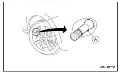
A Tyre valve with sensor
