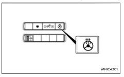
Push the heated steering wheel switch to warm the steering wheel after the hybrid system starts.
