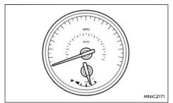
The speedometer indicates the vehicle speed. Scale resolution on the meter varies with models.
