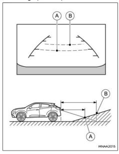
When reversing a vehicle up a hill, the distance guide lines and the vehicle width guide lines are shown closer than the actual distance. For example, the display shows 1 m (3 ft) to the place (A), but the actual 1 m (3 ft) distance on the hill is the place
