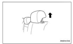
To raise the head restraint, pull it up as shown.
