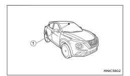
The Traffic Sign Assist (TSA) system provides the driver with information about the most recently detected speed limit. The system captures the road sign information with the multi-sensing front camera unit (1) located on the windshield in front of the interior rear-view mirror and displays the detected signs in the Vehicle Information Display.
