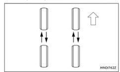
NISSAN recommends that tyres be rotated every 10,000 km (6,000 miles) for Two-Wheel Drive (2WD) vehicles and 5.000 km (3.000 miles) for Four-Wheel Drive (4WD) vehicles.
