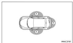
The Intelligent Key functions can only be used when the Intelligent Key is within the specified operating range from the request (lock/unlock) button ①.
