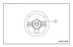
To sound the horn, push the centre pad area ① of the steering wheel.
