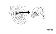
A Tyre valve with sensor
