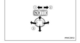
Slide the control to the left ① or to the right ② to select the left or right outside rear-view mirror,
