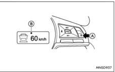
To turn the cruise control on, quickly push and release the Drive Assist switch A. A popup
