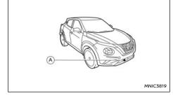
The sensor for the ICC system is located at the front of the vehicle A.
