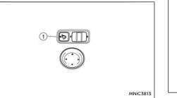
The outside rear-view mirrors fold when the outside rear-view mirror folding button (1) is pressed. To unfold, push the button again.
