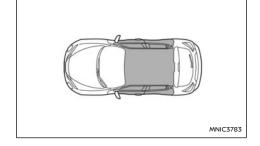
The Intelligent Key can only be used for starting the engine when the Intelligent Key is within the specified operating range (f) as illustrated.
