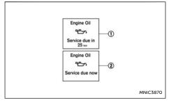
When the ignition is in the **ON** position, engine oil information is displayed.
