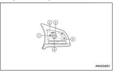
Each time the ICC system is turned on using the blue ProPILOT Assist switch (5), the distance setting reverts to [Long].
