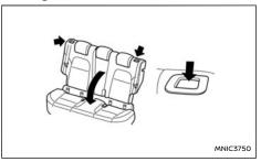
The luggage compartment loading capacity can be increased by folding the rear seats forward as shown.
