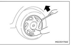
Removing wheel cover (where fitted)
