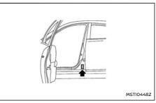
The cold tyre pressure is shown on the tyre placard fixed to the side of the driver's side centre pillar.
