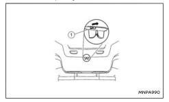
The vehicle's tailgate can be unlocked from the inside when the battery is dead. Tilt the seatback down. Slide the release lever ① as illustrated. See "Rear seats" (P.19) for more information regarding the seat operation.
