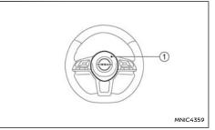
To sound the horn, push the centre pad area (1) of the steering wheel.
