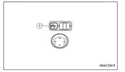
The outside rear-view mirrors fold when the outside rear-view mirror folding button (1) is pressed. To unfold, push the button again.
