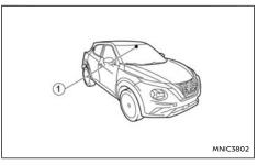
The lane camera unit ① for the Intelligent Lane Intervention system is located above the interior rear view mirror. To maintain the proper operation of the Intelligent Lane Intervention system and prevent a system malfunction, be sure to observe the following:
