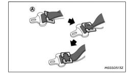
Route the seat belt tongue through the child restraint system and insert it into the buckle until you hear and feel the latch engage.
