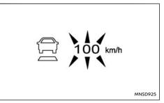
The driver can override ICC by pressing the accelerator. The set speed indicator will flash when the vehicle speed exceeds the set speed. The vehicle detect indicator will turn off when the area ahead of the vehicle is clear. When the pedal is released, the vehicle will return to the previously set speed.
