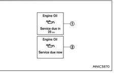
When the ignition is in the **ON** position, engine oil information is displayed.
