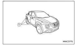
To display the multiple views, the IAVM system uses cameras 1 located in the front grille, on the vehicle's outside mirrors and one just above the vehicle's number plate. Do not put anything on the cameras.
