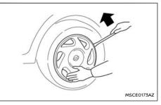
Removing wheel cover (where fitted)
