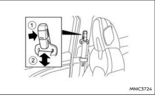
The shoulder belt anchor height should be adjusted to the position that is best for you. (See "Precautions on seat belt usage" (P.22).)
