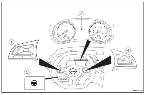
Steering Assist system controls (manual transmission vehicles)
