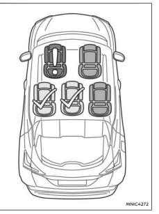
In addition to the Seat Belt Warning Light, the Occupant Status Display will be shown in the Vehicle Information Display (See "Vehicle information display" (P.67)) when any vehicle occupant's seat belt is not fastened.
