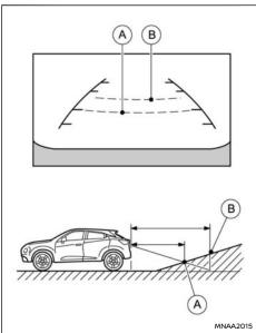
When reversing a vehicle up a hill, the distance guide lines and the vehicle width guide lines are shown closer than the actual distance. For example, the display shows 1 m (3 ft) to the place (a), but the actual 1 m (3 ft) distance on the hill is the place (a). Note that any object on the hill is viewed in the monitor further than it appears.
