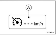
When pushing the Drive Assist switch on, the conventional (fixed speed) cruise control mode display and indicators are displayed in the vehicle information display. After you hold the Drive Assist switch for longer than about 1.5 seconds, the ICC system display goes out. The cruise indicator appears. You can now set your desired cruising speed. Pushing the Drive Assist switch again will turn the system completely off.
