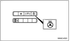
Push the heated steering wheel switch to warm the steering wheel after the engine starts.
