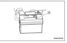
For a maintenance free battery it is not required to check the fluid level. However, NISSAN recommends to visually check the green indicator status periodically. If it is not visible, replace the battery as soon as possible.
