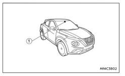
The lane camera unit ① for the LDW system is located above the interior rear view mirror. To maintain the proper operation of the LDW system and prevent a system malfunction, be sure to observe the following:
