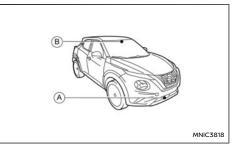
The IEB system uses a radar sensor  $\textcircled{}{}$  located at the front of the vehicle and a camera installed behind the windscreen  $\textcircled{}{}$  to measure the distance to the vehicle ahead in the travelling lane.
