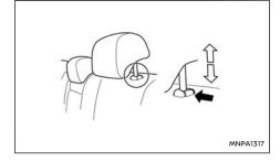
Align the head restraint stalks with the holes in the seat. Make sure that the head restraint is facing the correct direction. The stalk with the adjustment notch must be installed in the hole with the lock knob.
