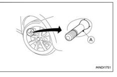
A Tyre valve with sensor
