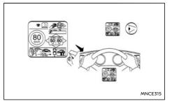
4. Remove the speed restriction sticker from the compressor, then place it in a location where the driver can see it while driving.
