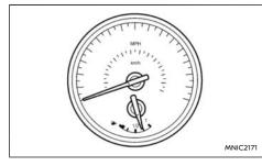
The speedometer indicates the vehicle speed. Scale resolution on the meter varies with models.
