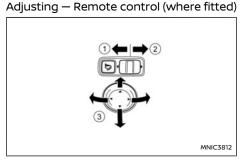
Slide the control to the left (1) or to the right (2) to select the left or right outside rear-view mirror,
