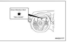
If the system detects that driver fatigue increases or that driver attention is decreasing, the message [Take a break?] appears in the Vehicle Information Display and a chime sounds when the vehicle is driven at speeds above 60 km/h (37 MPH).
