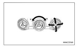
Adjust the air flow direction of the vents by opening, closing or rotating.
