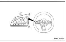
Switches for the trip computer are located on the left side of the steering wheel  $\triangle$ . To operate the trip computer, push the switches as shown above.
