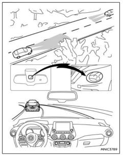
A camera-controlled high beam assistant which changes from low beam to high beam automatically.
