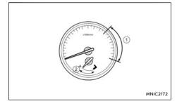
The tachometer indicates the engine speed in revolutions per minute. **Do not rev the engine into the red zone** ①.
