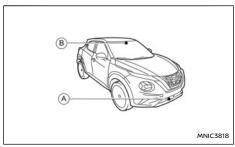
The sensor (A) is located behind the front bumper. The camera (B) is located on the upper side of the windscreen.
