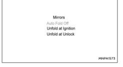
The outside rear-view mirrors automatically unfold when the ignition is switched on or when the vehicle doors are unlocked. Use the [Mirrors] menu of the Vehicle Information Display to select the moment that the mirrors are to be automatically folded and unfolded. The Auto fold feature can also be switched off. See "[Mirrors]" (P.72).
