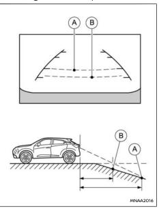
When reversing the vehicle down a hill, the distance guide lines and the vehicle width guide lines are shown further than the actual distance. For example, the display shows 1 m (3 ft) to the place (B, but the actual 1 m (3 ft) distance on the hill is the place (B. Note that any object on the hill is viewed in the monitor closer than it appears.
