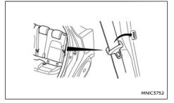
belts can be stored out of the way using the storage holder shown in the illustration.
