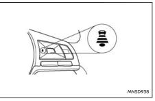
The distance to the vehicle ahead can be selected at any time depending on the traffic conditions.
