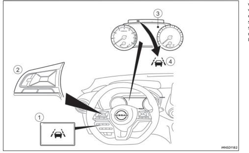
When the vehicle approaches either the left or the right side of the travelling lane, the steering wheel will vibrate and the ILI indicator (yellow) on the vehicle information display will blink to alert the driver. Then, the Intelligent Lane Intervention system will automatically apply the brakes for a short period of time to help assist the driver to return the vehicle to the centre of the travelling lane.
