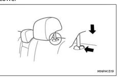
To lower, push and hold the lock knob and push the head restraint down as shown.
