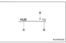
The clock (1) and outside air temperature (2) are displayed on the upper side of the Vehicle Information Display.
