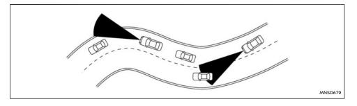
When driving on some roads, such as winding, hilly, curved, narrow roads, or roads which are under construction, the radar sensor may detect vehicles in a different lane, or may temporarily not detect a vehicle travelling ahead. This may cause the radar system to decelerate or accelerate the vehicle.
