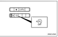
The system can be temporarily disengaged by pressing the Stop/Start System OFF switch. Pressing the button a second time will re-engage the Stop/Start System.
