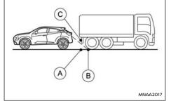
The position  $\bigcirc$  is shown further than the position B in the display. However, the position C is actually at the same distance as the position A. The vehicle may hit the object when moving toward the position A if the object projects over the actual moving course.
