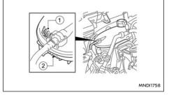
Check the coolant level in the reservoir when the engine is cold. If the coolant level is below MIN level (2), add coolant up to the MAX level (1). If the reservoir is empty, check the coolant level in the radiator **when the engine is cold**. If there is insufficient coolant in the radiator, fill the radiator with coolant up to the filler opening and also add it to the reservoir up to the MAX level (1).
