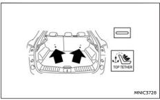
Anchor points are located on the seatback behind the rear outer seating positions and should only be used for child restraints in the rear outer positions. CHILD RESTRAINT INSTALLATION USING ISOFIX
