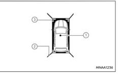
The bird's-eye view shows the overhead view of the vehicle, which helps confirm the vehicle position and the predicted course to a parking space. The vehicle icon ① shows the position of the vehicle.
