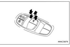
The automatic operation is available for the switch that has an  $|\mathbf{A}|$  mark on its surface.
