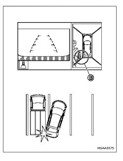
There may be a small visible distance between the vehicle and the object in the bird's-eye view B on the monitor.
