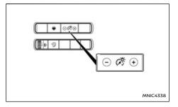
The instrument brightness control switch can be operated when the ignition is in the **ON** position. When the switch is operated, the brightness adjustment mode appears at the bottom of the vehicle information display.
