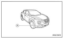
The radar sensor is located on the front of the vehicle  $\bigotimes$ .
