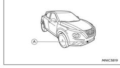
The sensor for the ICC system is located at the front of the vehicle  $\triangle$ .
