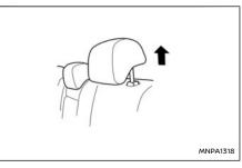
To raise the head restraint, pull it up as shown.
