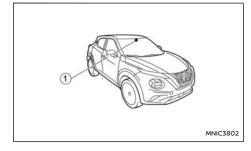
The sensor ① of the rain-sensing auto wiper system located on the upper part of the wind-screen, in front of the rear view mirror, can automatically turn on the wipers and adjust the wiper speed depending on the rainfall intensity and the vehicle speed when the lever in the <AUTO> position.
