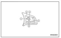
Push the ProPILOT Assist switch (5). This turns on the ProPILOT Assist system and displays the status of the ProPILOT Assist system on the Vehicle Information Display.
