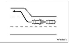
Pay attention to the driving operation to maintain control of the vehicle as it accelerates to the set speed. The ICC system does not control vehicle speed or warn you when you approach stationary and slow moving vehicles. You must pay attention to vehicle operation to maintain proper distance from vehicles ahead when approaching toll gates or traffic congestion.
