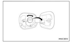
The fuel filler cap is a ratcheting type. Tighten the cap clockwise until ratcheting clicks are heard.
