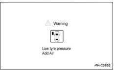
If you now press the **<OK>** switch on the steering wheel, a further screen is displayed to tell you the tyre pressure of all four tyres.
