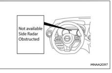
When radar blockage is detected, the system will be deactivated automatically. The [Not available Side Radar Obstructed] warning message will appear in the Vehicle Information Display.
