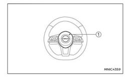
To sound the horn, push the centre pad area (1) of the steering wheel.
