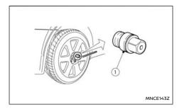
4. Loosen each wheel bolt by one or two turns anticlockwise with the wheel wrench.
