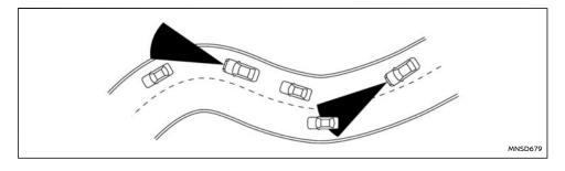
When driving on some roads, such as winding, hilly, curved, narrow roads, or roads which are under construction, the sensor may detect vehicles in a different lane, or may temporarily not detect a vehicle travelling ahead. This may cause the system to work inappropriately.
