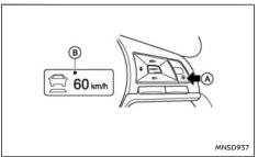
To turn the cruise control on, quickly push and release the Drive Assist switch A. A popup
