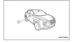
The lane camera unit ① for the LDW system is located above the interior rear view mirror. To maintain the proper operation of the LDW system and prevent a system malfunction, be sure to observe the following:
