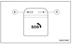
The indicator lights ④ and ⑤ above the **<SOS>** button indicate the status of the vehicle emergency call system. If the indicator light is illuminated red or no indicator light is illuminated the emergency call may not connect to the emergency call centre when the **<SOS>** button is pressed. Also an automatic emergency call may not be sent when a collision occurs.
