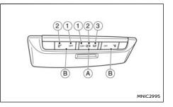
The room light (A) has a three-position switch.
