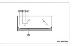
Guiding lines, which indicate the vehicle width and distances to objects with reference to the vehicle body line (A), are displayed on the monitor.
