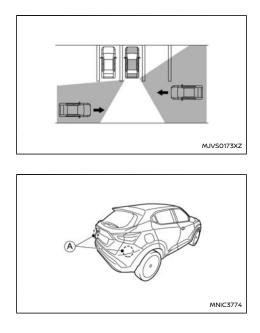
The RCTA system uses radar sensors (A) installed on both sides near the rear bumper to detect an approaching vehicle.
