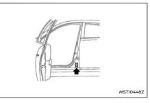
The cold tyre pressure is shown on the tyre placard fixed to the side of the driver's side centre pillar.
