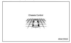
The automatic brake hold function status can be checked in the [Chassis Control] mode in the Vehicle Information Display. All four wheels will be highlighted when the system is active.
