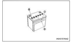
Check the fluid level in each cell. It should be between the UPPER 1 and LOWER 2 level lines.
