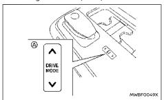
Use the Drive Mode Selector (A) located on the centre console to select the [ECO] mode. Use the [ECO] mode for maximum driving range and for city driving. The [ECO] mode helps reduce power consumption by reducing acceleration when compared to the same accelerator pedal position in the [STANDARD] mode. See "[ECO] mode" (P.280).
