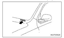
The vehicle identification number plate is attached as shown. This number is the identification for your vehicle and is used in the vehicle registration.
