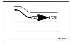
When driving on the highway at a vehicle set speed and approaching a slower travelling vehicle ahead, the ICC system adjusts the speed to maintain the distance, selected by the driver, from the vehicle ahead. If the vehicle ahead changes lanes or exits
