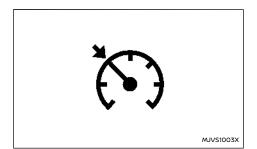
When the system is not operating properly, the chime sounds and the colour of the cruise indicator will change to yellow.
