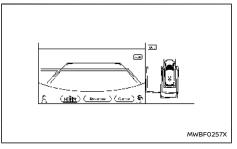
8. When the vehicle is in the parking guide box (light blue), the vehicle stops and parking control ends.
