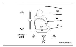
To defog/defrost the windscreen, start the EV system, display the climate control screen (see "Heater and air conditioner" (P.247)) and touch the heated windscreen key (A). Touch the key again to turn the system off.
