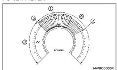
The power meter displays the traction motor power level when the accelerator pedal is depressed, as well as the level of power regeneration provided to the Li-ion battery by the regenerative brake
