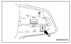
The distance to the vehicle ahead can be selected at the time of the ICC standby or the ICC is active.
