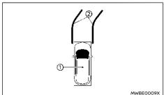
The bird's-eve view shows the overhead view of the vehicle which helps confirm the vehicle position and the predictive course to a parking space.
