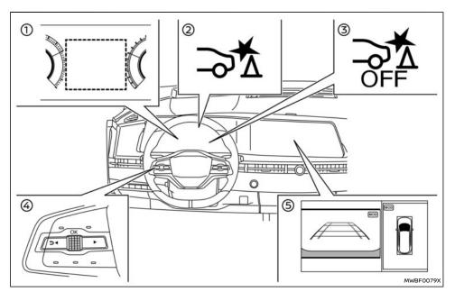
tion display, a red frame will appear in the centre display (models with the Intelligent Around View Monitor system), and the system will chime three times. The system will then automatically apply the brakes. After the automatic brake application, the driver must depress the brake pedal to maintain brake pressure.
