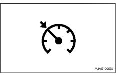
When the system is not operating properly, the chime sounds and the colour of the cruise indicator will change to vellow.
