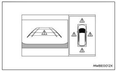
When the "  $\bigwedge$  " icon is displayed on the screen, there will be abnormal conditions in the Intelligent Around View Monitor This will not hinder normal driving operation but the system should be inspected. It is recommended you visit a NISSAN certified electric vehicle dealer.
