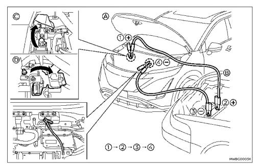
If the booster battery is in another vehicle (B), position the two vehicles (A) and (B) to bring their 12-volt batteries into close proximity to each other.
