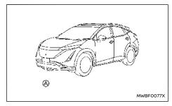
The radar sensor (A) is located on the front of the vehicle
