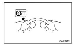
Take out the speed restriction sticker from the air compressor\*, then put it in a location where the driver can see it while driving.
