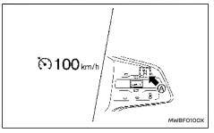
To turn on the conventional (fixed speed) cruise control mode, push and hold the Cruise ON/OFF switch (A) for longer than about 1.5 seconds.
