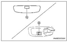
The inside mirror is designed so that it automatically changes reflection according to the intensity of the headlights of the following vehicle.
