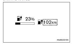
The driving range (km or miles) provides an estimated distance that the vehicle can be driven before recharging is necessary. The driving range is constantly being calculated, based on the amount of available Li-ion battery charge and the actual power consumption average.
