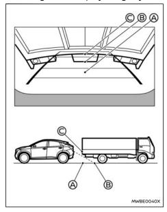
The position © is shown farther than the position ® in the display. However, the position © is actually at the same distance as the position ®. The vehicle may hit the object when reversing to the position ® if the object projects over the actual reversing course.
