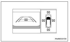
When the "\( \) " icon is displayed on the screen, the camera image may be receiving temporary electronic disturbances from surrounding devices. This will not hinder normal driving operation but the system should be inspected. It is recommended you visit a NISSAN certified electric vehicle dealer.
