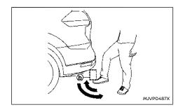
The liftgate can be operated using a quick kicking motion under the centre of the rear bumper.
