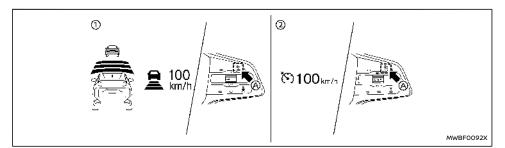
Selecting the vehicle-to-vehicle distance control mode To choose the vehicle-to-vehicle distance control mode ①, quickly push and release the Cruise ON/ OFF switch (A).
