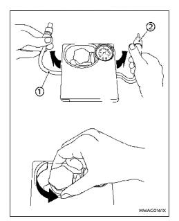
2. Take the hose (1) and the power plug (2) out of the air compressor. Remove the cap of the bottle holder from the air compressor.
