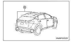
The BSW system uses radar sensors (A) installed near the rear bumper to detect other vehicles in an adjacent lane.
