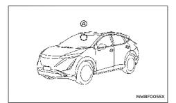
The Traffic Sign Recognition (TSR) system provides the driver with information about the most recently detected speed limit. The system captures the road sign information with the multi-sensing front camera unit (A) located on the windscreen in front of the inside mirror and displays the detected signs in the vehicle information display and in the Head Up Display (HUD) (where fitted). (See "Head Up Display (HUD) (where fitted)" (P.154).)
