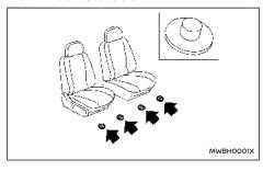
Your vehicle is equipped with floor mat positioning hook(s). The number and shape of the floor mat positioning hook(s) for each seating position varies depending on the vehicle.
