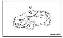
The ambient image sensor (A) for the high beam assist system is located in front of the inside mirror. To keep the proper operation of the high beam assist system and prevent a system malfunction, be sure to observe the following:
