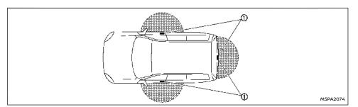
The Intelligent Key functions can only be used when the Intelligent Key is within the specified operating range from the lock or capacitive unlock sensors or the request switch (1).
