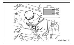
Check the fluid level in the reservoir. If the fluid is below the MIN line ②, the brake warning light will
