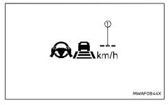
When the CANCEL switch is pushed down to the SET- direction under the following conditions, the ProPILOT Assist system cannot be set and the vehicle set speed indicator ① blinks for approximately 2 seconds:
