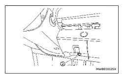
The sensors ① and ② located on the instrument panel, help maintain a constant temperature. Do not put anything on or around the sensors.
