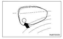
To open the charge port lid, unlock the doors (see "Intelligent Key system" (P.193)) and push the rear part of the lid as illustrated. Then open the charge port cap. (See "Charge port lid" (P.209).)
