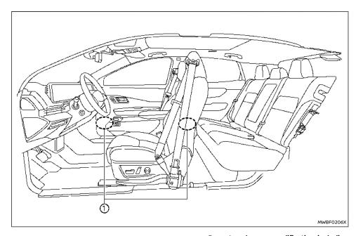
The active sound enhancement generates sounds according to motor speed and driving modes through the speakers ① to enhance the quality of the motor sound.
