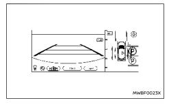
While the vehicle is stopped, check that (P) is displayed in the desired parking space.
