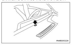
The charging status indicator light primarily indicates the charging status, and is visible from both inside and outside the vehicle.
