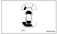
When the shift lever is in the R (Reverse) position and the Parking Aids screen is displayed in the vehicle information display the RAB system can be disabled temporarily by pushing the scroll dial on the steering wheel.
