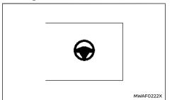
The Steering Assist switch, located on the driver's side instrument panel, is used to temporarily turn on and off the Steering Assist system.
