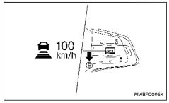
To set cruising speed, accelerate your vehicle to the desired speed, push the CANCEL switch to the SET- direction (B) and release it. (The ICC system ON indicator (green), set distance indicator and set vehicle speed indicator come on.) Take your foot off the accelerator pedal. Your vehicle will maintain the set speed.
