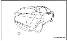
To display the rear view, the rear view monitor system uses a camera (1) located just above the vehicle's number plate.
