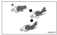
Route the seat belt tongue through the child restraint and insert it into the buckle until you hear and feel the latch engage. To prevent slack in the lap belt, secure the shoulder belt in place with a locking clip (a). Use a locking clip attached to the child restraint, or one which is equivalent in dimensions and strength.
