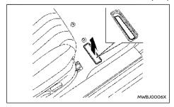
The vehicle identification number is located as shown.
