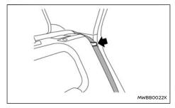
When folding down the rear seats, hook the rear outer seat belts on the seat belt hooks.
