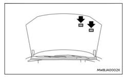
The air conditioner specification label(s) are attached to the underside of the bonnet as shown.
