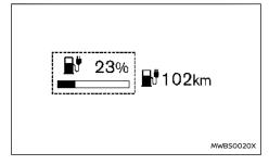
This indicator displays the available Li-ion battery power remaining to drive the vehicle.
