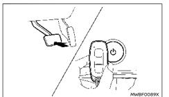
If the battery of the Intelligent Key is discharged, or environmental conditions interfere with the Intelligent Key operation, start the EV (Electric Vehicle) system in the READY to drive mode according to the following procedure:
