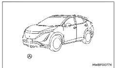
The sensor for the ICC system (A) is located on the front of the vehicle
