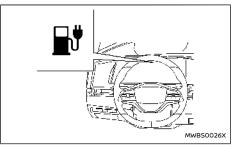
If the low battery charge warning light (yellow) illuminates, the Li-ion battery charge is too low for travel. See "Low battery charge warning light" (P.124). Charge the Li-ion battery as soon as possible.
