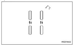
NISSAN recommends rotating the tyres at the specified interval shown in a separate maintenance booklet. (For tyre replacing procedures, see "Jacking up vehicle and replacing tyres" (P.472).)
