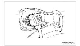
Follow the instructions on the quick charge equipment to start charging. When the equipment is properly installed and ready to charge, a beep sounds twice and the charging status indicator light will operate. See "Charging status indicator light" (P.53).
