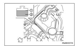
Check the coolant level in the reservoir when the high voltage parts are cold. If the coolant level is below the MIN level (2), open the reservoir cap and add coolant up to the MAX level (1). If the reservoir is empty, check the coolant level in the coolant tank when the high voltage parts are cold. If there is insufficient coolant in the coolant tank, fill the coolant tank with coolant up to the reservoir cap opening and also add it to the reservoir up to the MAX level (1).
