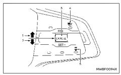
The system is operated by a Cruise ON/OFF switch and four control switches, all mounted on the steering wheel.
