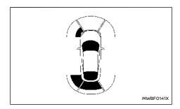
When the vehicle moves closer to an obstacle, the parking sensor indicator (detected area) appears in the vehicle information display.
