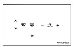
To defog/defrost the rear window glass and outside mirrors, start the EV system and push the switch on. The indicator light (A) will illuminate. Push the switch again to turn the defroster off.
