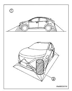
There are some areas where the system will not show objects and the system does not warn of moving objects. When in the front or the rear view display, an object below the bumper or on the ground may not be viewed 1. When in the bird'seye view, a tall object near the seam 2 of the camera viewing areas will not appear in the monitor.
