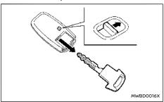
To remove the mechanical key, release the lock knob at the back of the Intelligent Key.
