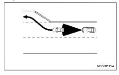
When driving on the highway at a vehicle set speed and approaching a slower travelling vehicle ahead, the ICC system adjusts the speed to maintain the distance, selected by the driver, from the vehicle ahead. If the vehicle ahead changes lanes or exits
