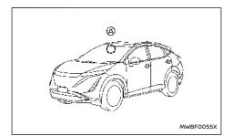
The Traffic Sign Recognition (TSR) system provides the driver with information about the most recently detected speed limit. The system captures the road sign information with the multi-sensing front camera unit (a) located on the windshield in front of the inside mirror and displays the detected signs in the vehicle information display and in the Head Up Display (HUD) (where fitted). (See "Head Up Display (HUD) (where fitted)" (P.152).)
