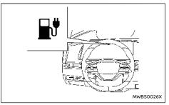
If the low battery charge warning light (yellow) illuminates, the Li-ion battery charge is too low for travel. See "Low battery charge warning light" (P.122). Charge the Li-ion battery as soon as possible.
