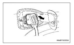
Remove the charge connector from the vehicle and store it away properly.
