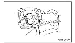
Follow the instructions on the quick charge equipment to start charging. When the equipment is properly installed and ready to charge, a beep sounds twice and the charging status indicator light will operate. See "Charging status indicator light" (P.51).
