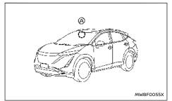
The ambient image sensor (A) for the adaptive LED headlight system is located in front of the inside mirror. To keep the proper operation of the adaptive LED headlight system and prevent a system malfunction, be sure to observe the following:
