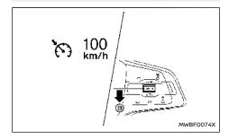
To set cruising speed, accelerate your vehicle to the desired speed, push down the CANCEL switch to the SET- (B) direction and release it. (The colour of the cruise indicator changes to green and vehicle set speed indicator comes on.) Take your foot off the accelerator pedal. Your vehicle will maintain the set speed.
