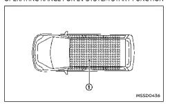
The Intelligent Key can only be used for starting the EV system when the Intelligent Key is within the specified operating range (1).
