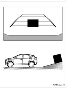
When reversing the vehicle up a hill, the distance guide lines and the vehicle width guide lines are shown closer than the actual distance. Note that any object on the hill is farther than it appears on the monitor.
