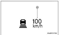
The driver can override ICC by depressing the accelerator pedal. The set speed indicator (A) will flash when the vehicle speed exceeds the set speed. The vehicle detect indicator will turn off when the area ahead of the vehicle is open. When the pedal is released, the vehicle will return to the previously set speed.
