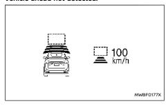
When a vehicle is no longer detected ahead, the ICC system gradually accelerates your vehicle to resume the previously set vehicle speed. The ICC system then maintains the set speed.
