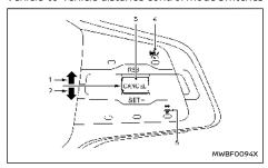
The system is operated by a Cruise ON/OFF switch and four control switches, all mounted on the steering wheel.
