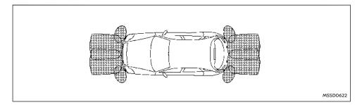
The parking sensor (sonar) system sounds a tone to inform the driver of obstacles near the bumper.
