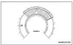
This meter displays the actual traction motor power consumption and the regenerative brake power provided to the Li-ion battery.
