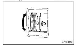
The headlight aiming control operates when the power switch is in the ON position and the headlight is on to allow the headlight axis to be adjusted according to the driving conditions.
