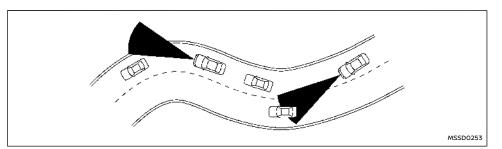
When driving on some roads, such as winding, hilly, curved, narrow roads, or roads which are under construction or on a slope, the sensor may detect vehicles in a different lane, or may temporarily not detect a vehicle traveling ahead. This may cause the system to work inappropriately.
