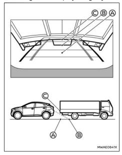
The position © is shown farther than the position (B) in the display. However, the position (C) is actually at the same distance as the position (A) . The vehicle may hit the object when reversing to the position (a) if the object projects over the actual moving course.
