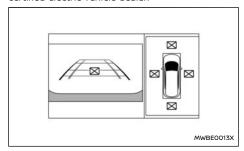
When the "\sum " icon is displayed on the screen, the camera image may be receiving temporary electronic disturbances from surrounding devices. This will not hinder normal driving operation but the system should be inspected. It is recommended you visit a NISSAN certified electric vehicle dealer.
