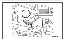
Check the fluid level in the reservoir. If the fluid is below the MIN line (2), the brake warning light will
