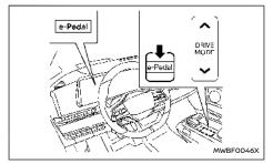
The e-Pedal Step system will be turned ON or OFF each time the <e-Pedal> switch (located on the centre console) is operated. (The e-Pedal Step indicator in the vehicle information display shows the status of the e-Pedal Step system.)
