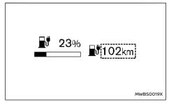
This indicator displays the estimated driving range (calculated based on a programme that accounts for current driving style and operational conditions) that can be driven before recharging is necessary.
