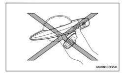
Do not use the lock or capacitive unlock sensors or the request switch with the Intelligent Key held in your hand as illustrated. The close distance to the door handle will cause the Intelligent Key system to have difficulty
