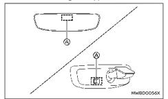
The inside mirror is designed so that it automatically changes reflection according to the intensity of the headlights of the following vehicle.
