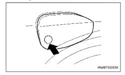
To open the charge port lid, unlock the doors (see "Intelligent Key system" (P.191)) and push the rear part of the lid as illustrated.
