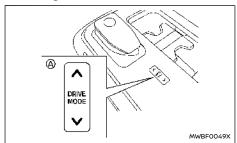
Use the Drive Mode Selector (A) located on the centre console to select the [ECO] mode. Use the [ECO] mode for maximum driving range and for city driving. The [ECO] mode helps reduce power consumption by reducing acceleration when compared to the same accelerator pedal position in the [STANDARD] mode. See "[ECO] mode" (P.276).
