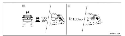
Selecting the vehicle-to-vehicle distance control mode To choose the vehicle-to-vehicle distance control mode ①, quickly push and release the Cruise ON/ OFF switch ⓐ.
