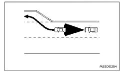
When driving on the freeway at a set speed and approaching a slower travelling vehicle ahead, the ICC system will adjust the speed to maintain the distance, selected by the driver, from the vehicle ahead. If the vehicle ahead changes lanes or exits the freeway, the ICC system will accelerate and maintain the speed up to the set speed. Pay attention to the driving operation to maintain control of the vehicle as it accelerates to the set speed.
