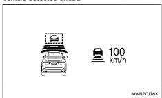
When a vehicle is detected in the lane ahead, the ICC system decelerates the vehicle by controlling the throttle and applying the brakes to match the speed of a slower vehicle ahead. The system then controls the vehicle speed based on the speed of the vehicle ahead to maintain the driver selected distance.
