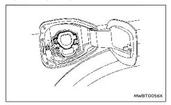
Normal charge can be performed either at home or at a public charging facility. There are two methods for performing normal charge. You can either connect the vehicle and the power supply to the EVSE (Electric Vehicle Supply Equipment) (where fitted), or connect the vehicle to a normal charger. NISSAN recommends using normal charge for usual charging of the vehicle. Use of quick charge should be minimised in order to prolong Li-ion battery life.
