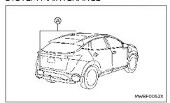
The two radar sensors (A) for the BSW system are located near the rear bumper. Always keep the area near the radar sensors clean.
