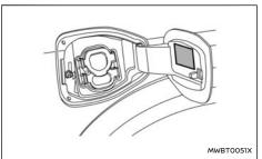
The vehicle charge port (back side of the lid) and/ or the charge connector may have an identifier which specifies the type of charging.
