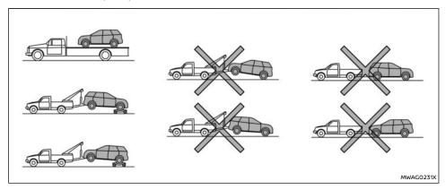
NISSAN recommends that towing dollies be used when towing your vehicle or the vehicle be placed on a flat bed truck as illustrated.
