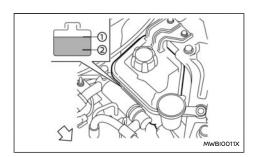
Check the coolant level in the reservoir when the high voltage parts are cold. If the coolant level is below the MIN level 2, open the reservoir cap and add coolant up to the MAX level (1). If the reservoir is empty, check the coolant level in the coolant tank when the high voltage parts are cold. If there is insufficient coolant in the coolant tank, fill the coolant tank with coolant up to the reservoir cap opening and also add it to the reservoir up to the MAX level (1).
