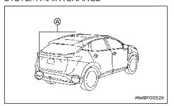
The two radar sensors (A) for the RCTA system are located near the rear bumper. Always keep the area near the radar sensors clean.
