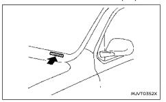
The vehicle identification number plate is attached
