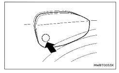
To open the charge port lid, unlock the doors (see "Intelligent Key system" (P.191)) and push the rear part of the lid as illustrated. Then open the charge port cap. (See "Charge port lid" (P.206).)
