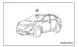
Be sure not to put anything on top of the sensor (A) located in front of the inside mirror. The sensor controls the Intelligent Auto Headlight; if it is covered, the sensor reacts as if it is dark and the headlights will illuminate.
