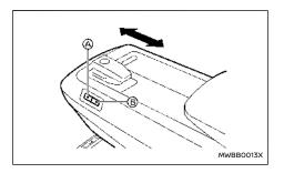
The position of the console box can be adjusted to your desired position.
