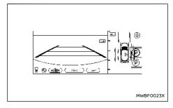
While the vehicle is stopped, check that (P) is displayed in the desired parking space.
