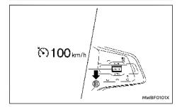
To set cruising speed, accelerate your vehicle to the desired speed, push the CANCEL switch to the SET- direction (a) and release it. (The colour of the cruise indicator changes to green and set vehicle speed indicator comes on.) Take your foot off the accelerator pedal. Your vehicle will maintain the set speed.
