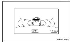
When the vehicle speed becomes approximately 10 km/h or higher while parking position detection is in progress, the screen changes. When the vehicle speed drops to approximately 10 km/h or less, the screen returns to the regular ProPILOT Park screen
