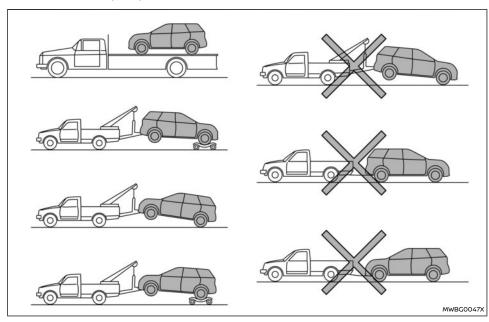
NISSAN recommends that your vehicle be towed with the driving (front) wheels off the ground or that the vehicle be placed on a flatbed truck as illustrated.
