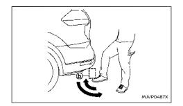
The liftgate can be operated using a quick kicking motion under the centre of the rear bumper.
