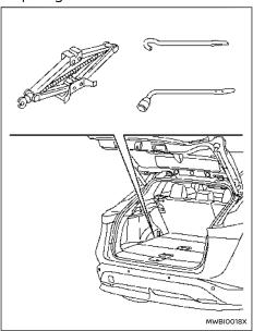
Open the liftgate. Raise the luggage floor board. Remove the jacking tools.
