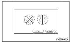
Depress the brake pedal and stop the vehicle, then touch the parking guide box adjustment icon (6) on the screen.
