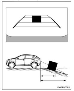
When reversing the vehicle down a hill, the distance guide lines and the vehicle width guide lines are shown farther than the actual distance. Note that any object on the hill is closer than it appears on the monitor.
