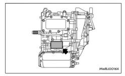
Rear traction motor (where fitted)
