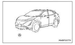
The Intelligent Forward Collision Warning system uses a radar sensor (A) located on the front of the vehicle to measure the distance to a second vehicle ahead in the same lane.
