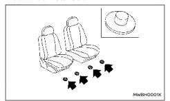
Your vehicle is equipped with floor mat positioning hook(s). The number and shape of the floor mat positioning hook(s) for each seating position varies depending on the vehicle.
