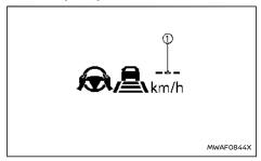
When the CANCEL switch is pushed down to the SET- direction under the following conditions, the ProPILOT Assist system cannot be set and the vehicle set speed indicator ① blinks for approximately 2 seconds:
