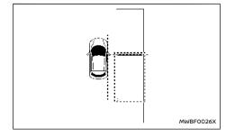
Drive slowly forward and depress the brake pedal to stop the vehicle when parallel to the parking position.
