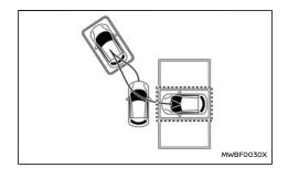
Parking control is performed using a route as shown in the illustration.
