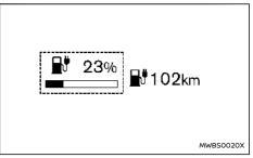
This indicator displays the available Li-ion battery power remaining to drive the vehicle.
