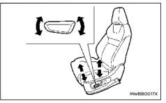
Move the switch as shown to adjust the angle of the front portion or height of the seat.
