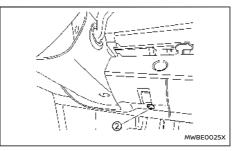
The sensors (1) and (2) located on the instrument panel, help maintain a constant temperature. Do not put anything on or around the sensors.
