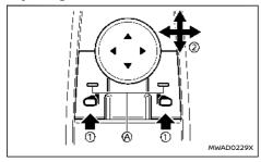
The outside mirror control switch is located on the driver's armrest.
