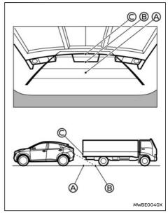
The position O is shown farther than the position O is actually at the same distance as the position O. The vehicle may hit the object when reversing to the position O if the object projects over the actual reversing course.
