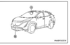
The radar sensor B is located on the front of the vehicle. The camera A is located on the upper side
