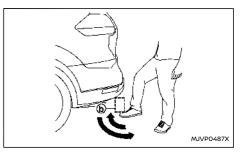
The liftgate can be operated using a quick kicking motion under the centre of the rear bumper.
