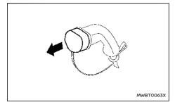
6. Remove the safety cap (where fitted) from the normal charge connector.
