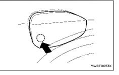
To open the charge port lid, unlock the doors (see "Intelligent Key system" (P.182)) and push the rear part of the lid as illustrated. Then open the charge port cap. (See "Charge port lid" (P.197).)
