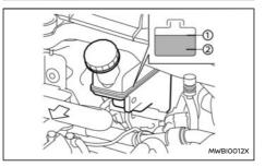
Check the fluid level in the reservoir. If the fluid is below the MIN line (2), the brake warning light will
