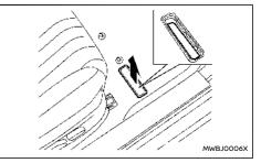
The vehicle identification number is located as shown.
