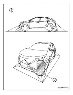
There are some areas where the system will not show objects and the system does not warn of moving objects. When in the front or the rear view display, an object below the bumper or on the ground may not be viewed ①. When in the bird'seye view, a tall object near the seam ② of the camera viewing areas will not appear in the monitor.
