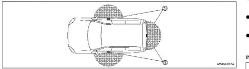
The Intelligent Key functions can only be used when the Intelligent Key is within the specified operating range from the lock or capacitive unlock sensors or the request switch (1).
