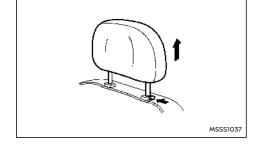
Use the following procedure to remove the head restraint.
