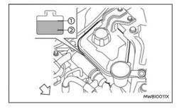
Check the coolant level in the reservoir when the high voltage parts are cold. If the coolant level is
