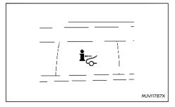
To turn the HUD on, push the HUD switch. To turn the HUD off, push the switch again.
