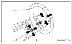
Move the lever (f) to adjust the steering wheel up or down, forward or rearward until the desired position is achieved.
