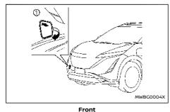
Make sure that the recovery hook is properly secured in its storage area after use.
