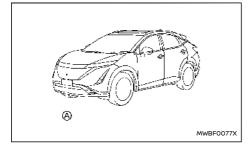
The radar sensor  $\textcircled{\ensuremath{\mathbb A}}$  is located on the front of the vehicle.
