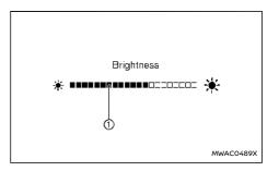
The instrument brightness control switch can be operated when the power switch is in the ON position. When the switch is operated, the vehicle information display switches to the brightness adjustment mode.
