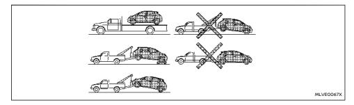
NISSAN recommends that your vehicle be towed with the driving (front) wheels off the ground or that the vehicle be placed on a flatbed truck as illustrated.
