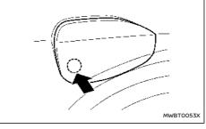
To open the charge port lid, unlock the doors then push the part of the lid near the rear of the vehicle (Refer to the figure).
