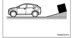
When reversing the vehicle up a hill, the distance guide lines and the vehicle width guide lines are shown closer than the actual distance. Note that any object on the hill is farther than it appears on the monitor.
