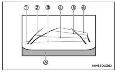
Guiding lines which indicate the vehicle width and distances to objects with reference to the bumper line A are displayed on the monitor.
