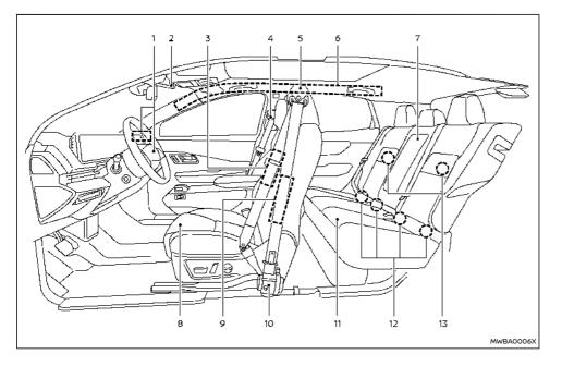
13. Child restraint anchor points (for top tether strap) (P.78)
