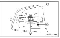
The vehicle information display can be changed using the dial/buttons located on the steering wheel.
