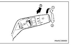
The rear window wiper and washer operate when the power switch is in the ON position.
