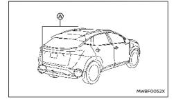
The two radar sensors (A) for the RCTA system are located near the rear bumper. Always keep the area near the radar sensors clean.
