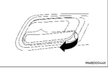
To unlock and open the door, pull the inside door handle as illustrated.
