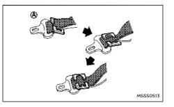
Route the seat belt tongue through the child restraint and insert it into the buckle until you hear and feel the latch engage.
