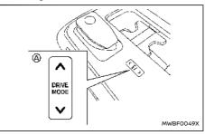
Use the Drive Mode Selector (A) located on the centre console to select the ECO mode. Use the ECO mode for maximum driving range and for city driving. The ECO mode helps reduce power consumption by reducing acceleration when compared to the same accelerator pedal position in the STANDARD mode. See "ECO mode" (P.265).
