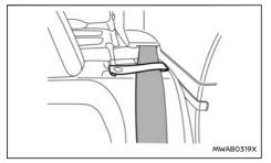
When the seat belt guide is used on the rear seat, the seat belt can easily be pulled out. Do not allow the seat belt to twist.
