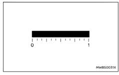
This gauge displays the available capacity of the Li-ion battery remaining to store power.
