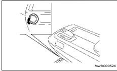
Before inserting or disconnecting a plug, be sure the electrical accessory being used is turned OFF.
