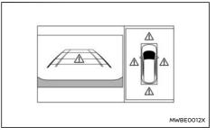
When the "  $\bigwedge$  " icon is displayed on the screen, there will be abnormal conditions in the Intelligent Around View Monitor. This will not hinder normal driving operation but the system should be inspected. It is recommended you visit a NISSAN certified electric vehicle dealer.
