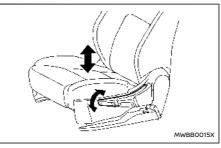
Pull up or push down the adjusting lever to adjust the seat height until the desired position is achieved.
