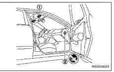
Warning labels about the supplemental air bag system are placed in the vehicle as shown in the illustration. The warning label ① is located on the surface of the driver's and/or passenger's sun visor.
