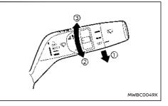
The rain-sensing auto wiper system can automatically turn on the wipers and adjust the wiper speed depending on the rainfall and the vehicle speed by using the rain sensor located on the upper part of the windscreen.
