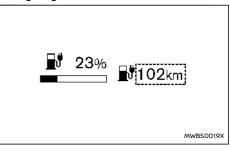
This indicator displays the estimated driving range (calculated based on a programme that accounts for current driving style and operational conditions) that can be driven before recharging is necessary.
