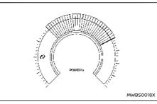
This meter displays the actual traction motor power consumption and the regenerative brake power provided to the Li-ion battery.
