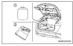
Take out the emergency tyre puncture repair kit from the storage area under the luggage floor board. The repair kit consists of the following items:
