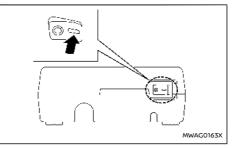
6. Place the power switch in the ON position. Then turn the compressor switch to the ON (-) position and inflate the tyre up to the pressure that is specified on the tyre placard affixed to the driver's side centre pillar if possible, or to the minimum of 180 kPa (26 psi). Turn the air compressor off briefly in order to check the tyre pressure with the pressure gauge.
