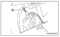
When taking out or putting away the storage bag, remove hook A from the anchor. When the NISSAN Mode 3 cable (where fitted) is stored, be sure to fasten the hook in place securely.
