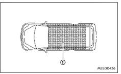
The Intelligent Key can only be used for starting the electric vehicle system when the Intelligent Key is within the specified operating range ①.
