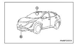
The Intelligent Emergency Braking system uses a radar sensor B located on the front of the vehicle to measure the distance to the vehicle ahead in the same lane.
