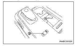
To open the flexible centre storage, push and hold the OPEN side of the switch A located on the
