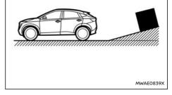
When reversing the vehicle up a hill, the distance guide lines and the vehicle width guide lines are shown closer than the actual distance. Note that any object on the hill is farther than it appears on the monitor.
