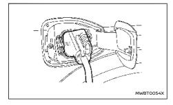
Follow the instructions on the quick charge equipment to start charging. When the equipment is properly installed and ready to charge, a beep sounds twice and the charging status indicator light will operate. See "Charging status indicator light" (P.49).
