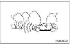
The Approaching Vehicle Sound for Pedestrians (VSP) system is a function that uses sound to alert pedestrians of the presence of the vehicle when it is being driven at a low speed.
