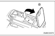
To open the console box lid, pull up the lid while pushing the button A at the inside of the lid.
