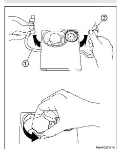
Take the hose ① and the power plug ② out of the air compressor. Remove the cap of the bottle holder from the air compressor.
