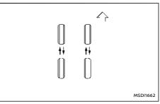
NISSAN recommends rotating the tyres at the specified interval shown in the maintenance schedule. (For tyre replacing procedures, see "Jacking up vehicle and replacing tyres" (P.460).) As soon as possible, tighten the wheel nuts to the specified torque with a torque wrench.
