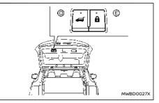
Power liftgate close and lock switches - Liftgate
