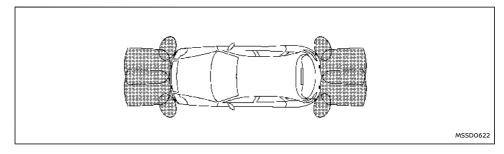
The parking sensor (sonar) system sounds a tone to inform the driver of obstacles near the bumper.
