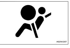
The supplemental air bag warning light, displaying rin the meter monitors the circuits for the air bag systems, pre-tensioner seat belt system and all related wiring.
