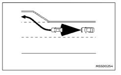
When driving on the freeway at a set speed and approaching a slower travelling vehicle ahead, the ICC system will adjust the speed to maintain the distance, selected by the driver, from the vehicle ahead. If the vehicle ahead changes lanes or exits the freeway, the ICC system will accelerate and maintain the speed up to the set speed. Pay attention to the driving operation to maintain control of the vehicle as it accelerates to the set speed.
