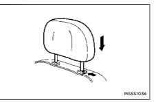
To lower, push and hold the lock knob and push the head restraint down.
