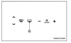
To defog/defrost the rear window glass and outside mirrors, start the electric vehicle system and push the switch on. The indicator light A will illuminate. Push the switch again to turn the defroster off.
