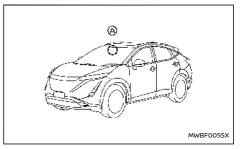
The lane camera unit (A) for the Intelligent Lane Intervention system is located above the inside mirror. To keep the proper operation of the Intelligent Lane Intervention system and prevent a system malfunction, be sure to observe the following:
