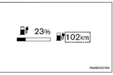
The driving range (km or miles) provides an estimated distance that the vehicle can be driven before recharging is necessary. The driving range is constantly being calculated, based on the amount of available Li-ion battery charge and the actual power consumption average.
