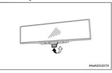
The mode can be switched when the power switch is in the ON position.
