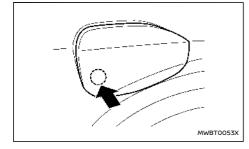
To open the charge port lid, unlock the doors (see "Intelligent Key system" (P.182)) and push
