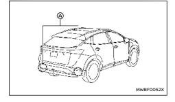
The BSW system uses radar sensors (A) installed near the rear bumper to detect other vehicles in an adjacent lane.
