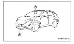
The camera (a) is located above the inside mirror. The front radar sensor (B) is located on the front of the vehicle. To keep the ELA system operating properly, be sure to observe the following:
