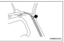
When folding down the rear seats, hook the rear outer seat belts on the seat belt hooks.
