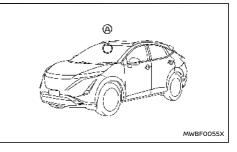
The ambient image sensor (A) for the high beam assist system is located in front of the inside mirror. To keep the proper operation of the high beam assist system and prevent a system mal-function, be sure to observe the following:
