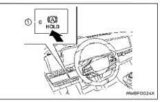
With the power switch in the ON position, push the automatic brake hold switch. The indicator light ① on the automatic brake hold switch illuminates.  When the automatic brake hold function goes into standby, the automatic brake hold indicator light (white) illuminates.
