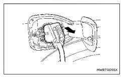
2. Remove the charge connector from the vehicle and store it away properly.
