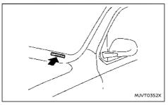
as shown. This number is the identification for your vehicle and is used in the vehicle registration.
