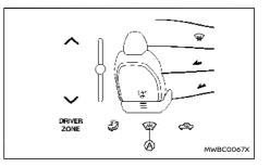
To defog/defrost the windscreen, start the electric vehicle system, display the climate control screen (see "Heater and air conditioner" (P.235)) and touch the heated windscreen key (A). Touch the key again to turn the system off.
