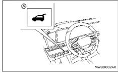
Power liftgate switch - Instrument panel
