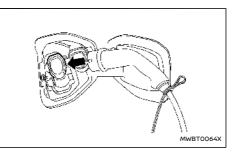
Connect the charge connector to the charge port. If it is connected normally, a beep will sound once.
