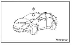
The ambient image sensor (A) for the adaptive LED headlight system is located in front of the inside rearview mirror. To keep the proper operation of the adaptive LED headlight system and prevent a system malfunction, be sure to observe the following:
