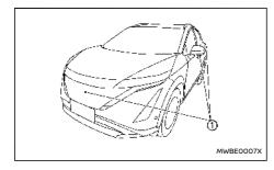
To display the multiple views, the Intelligent Around View Monitor system uses cameras (1) located on the front grille, on the vehicle's outside mirrors and one just above the vehicle's rear number plate.
