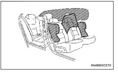
The supplemental side-impact air bag is located at the outside of the front seats' seatbacks.
