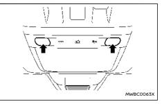
Touch the light to turn the map light on. To turn the light off, touch the light again.
