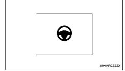
The dynamic driver assistance switch, located on the driver's side instrument panel, is used to temporarily turn on and off the Intelligent Lane Intervention system and Intelligent Blind Spot Intervention system (where fitted).
