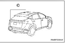
The two rear radar sensors (C) for the ELA system are located near the rear bumper. Always keep the area near the radar sensors clean.
