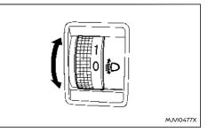
The headlight aiming control operates when the power switch is in the ON position and the headlight is on to allow the headlight axis to be adjusted according to the driving conditions.
