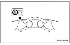
Take out the speed restriction sticker from the air compressor\*, then put it in a location where the driver can see it while driving.
