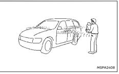
Do not use the lock or capacitive unlock sensors or the request switch with the Intelligent Key held in your hand as illustrated. The close distance to the door handle will cause the Intelligent Key system to have difficulty recognising that the Intelligent Key is outside
