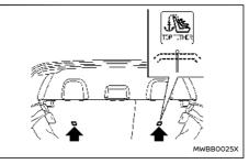
Anchorages are located as illustrated. Position the top tether strap over the top of the seatback and secure it to the tether anchorage that provides the straightest installation. Tighten the tether strap according to the manufacturer's instruction to remove any slack.
