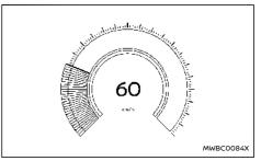
The speedometer indicates vehicle speed (km/h or MPH).
