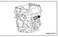
The vehicle identification number plate is attached
