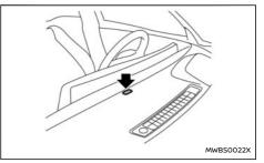
The charging status indicator light primarily indicates the charging status, and is visible from both inside and outside the vehicle.
